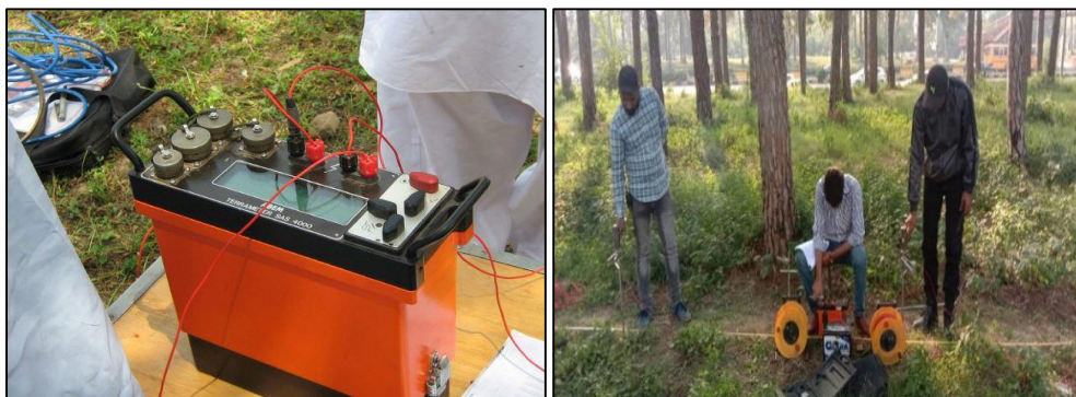
Figure.3.3 Setting of Potential and Current Electrodes
