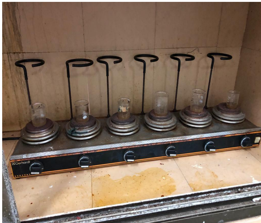
Figure 2. Acid Digestion of soil samples, oven drying and heating on hot plates with nitric acid and perchloric acid.
