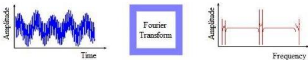
Figure 12 : The general practice in time series signal measurement is known as Fourier transforms (FT).
