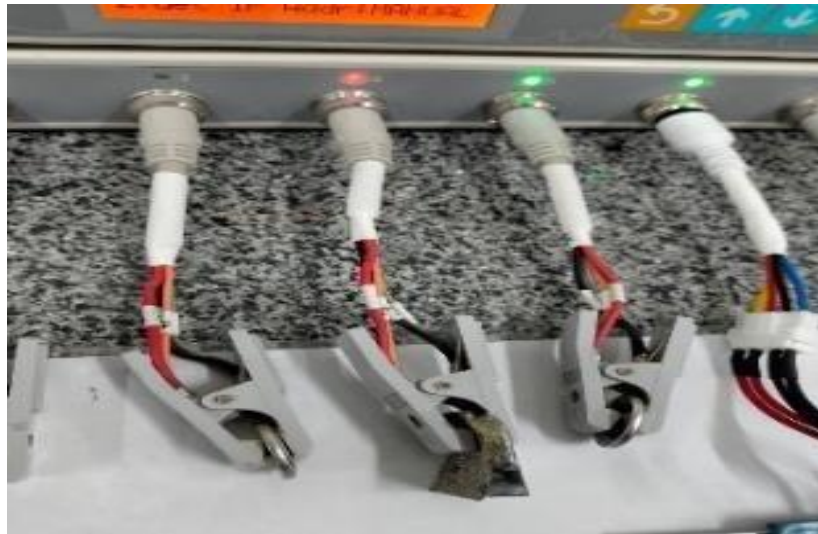
Figure 15: Evaluation of Battery in NEWARE testing unit.
