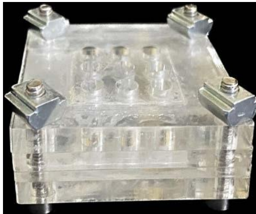
Figure 8: Battery Assembled in Casing.
