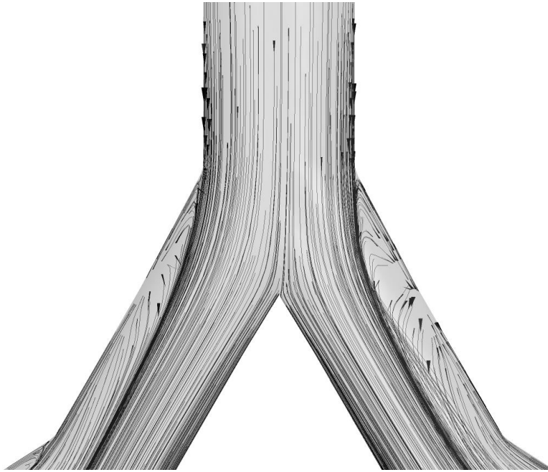
Figure 10: Separation of streamlines and generation of secondary vortices on the symmetric plane at the bifurcation region of G3.
