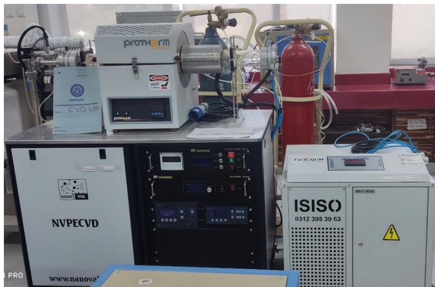
Figure 3-9. Plasma Enhanced Chemical Vapor Deposition (NVPECVD).
