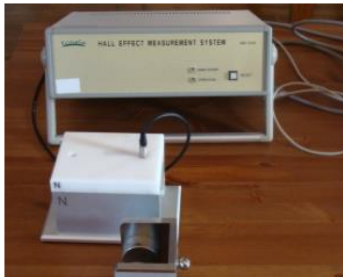
Figure 3-26. Hall Effect Measurement System (HMS-3000).
