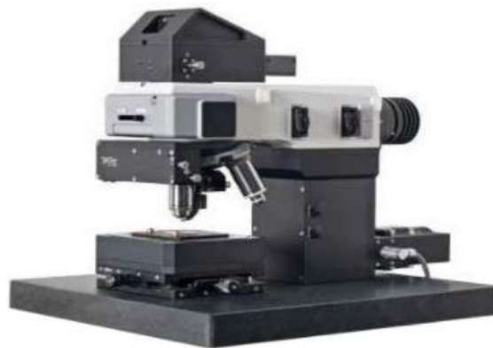
Figure 3-22. Atomic Force Microscopy (Model: Alpha 300 A).
