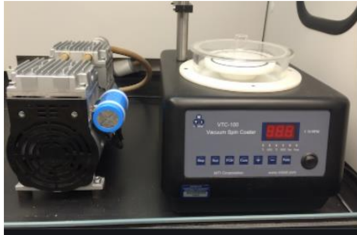
Figure 3-2. Vacuum Spin coater (VTC-100PA).
