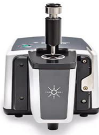
Figure 3-18. Fourier Transform Infrared Spectroscopy (Cary-630).
