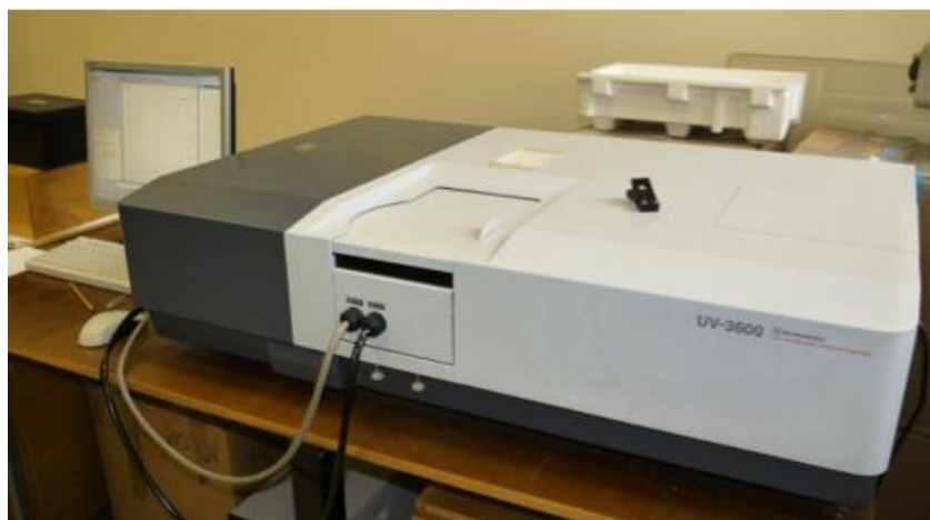
Figure 3-24. UV-Vis-NIR Spectrophotometry (3600-PLUS).
