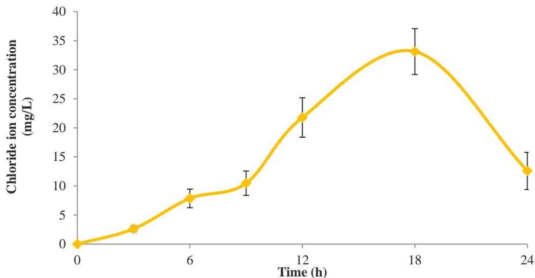
**Figure 4.31: Change in concentration of chloride ions during CP biodegradation in mineral salt medium at pH7 and inoculated with MCs.**
