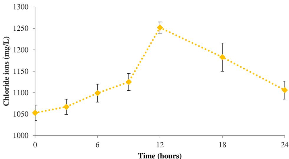
**Figure 4.18: Change in concentration of chloride ions during CP biodegradation in WW (CP 545 mg/L; pH 7; HRT 24 h; Glucose 2 g/L)**
