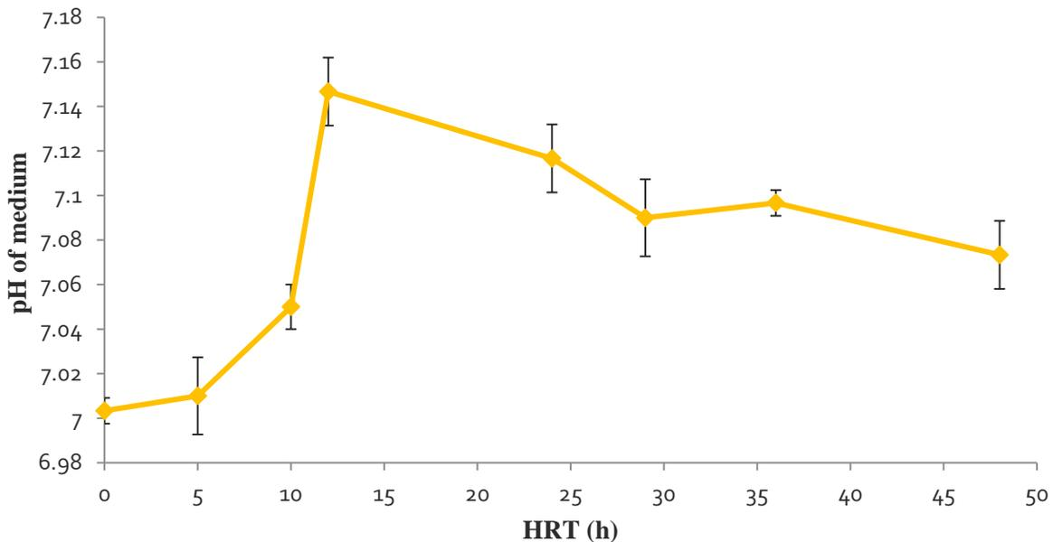
**Figure 4.9:** Fluctuation of pH during CP biodegradation in mineral salt medium supplemented with initial CP concentration; 400 mg/L, initial pH; 7, HRT; 48 h.
