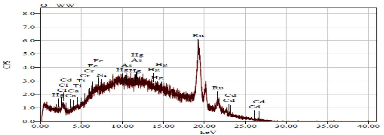
**Figure II a:** XRF pattern of two wastewater samples (1) collected from agrochemical industry for various metals (voltage; 30Kv, Current; 1mA, Energy range; 0 - 41KeV, Counting rate; 10565counts/sec).
