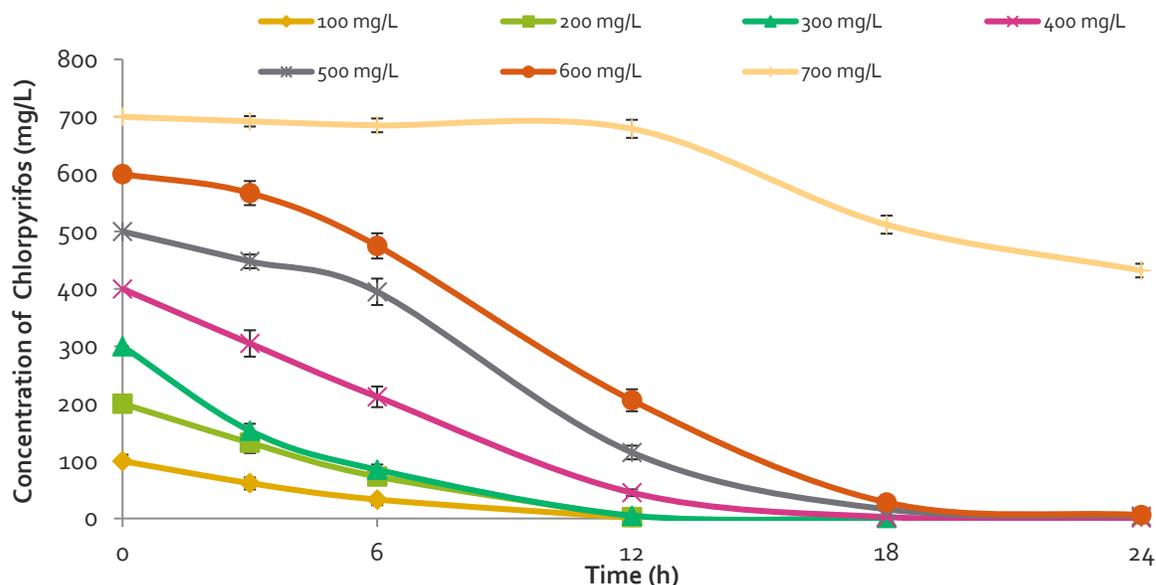
**Figure 4.26: Biodegradation of CP using macrocapsules (encapsulation bacterial consortium) at varying initial CP concentration from 100 to 700 mg/L in MSM at pH 7 and incubation time 24 h.**
