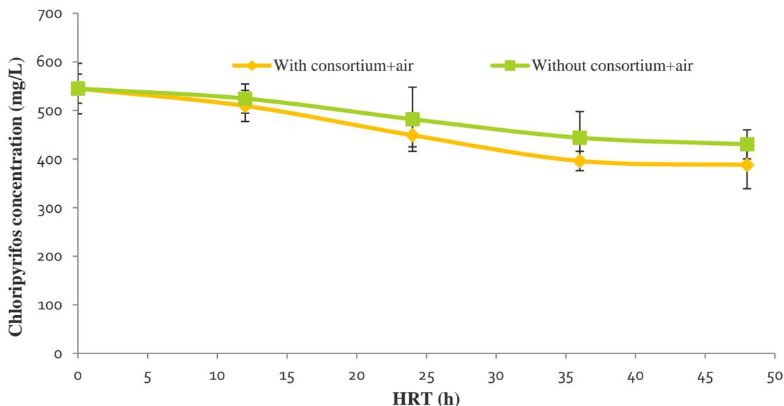
**Figure 4.13: Biodegradation of CP in WW when bacterial consortium was used as seeding inoculum initial CP concentration 545 mg/L; hydraulic retention time; 48 h.**
