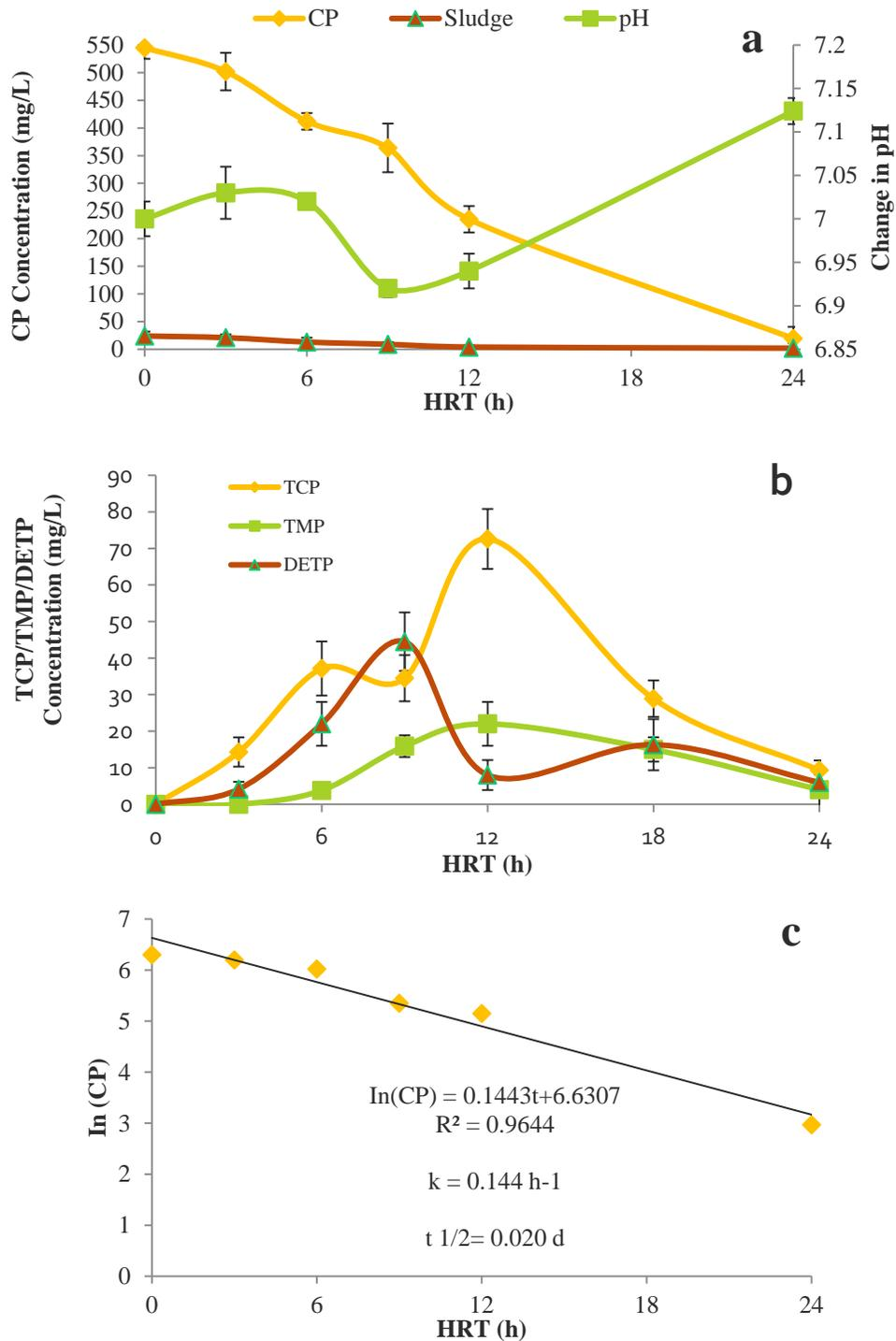
**Figure 4.16: Biodegradation of CP in WW (a) CP concentration and pH (b) concentration of metabolites (c) change in  $\ln(\text{CP})$  with time (CP; 545 mg/L, Ph; 7, HRT; 24 h, Glucose; 2 g/L)**
