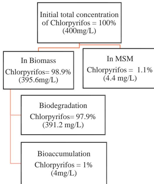
**Figure 4.10: Removal mechanism and mass balance of CP biodegradation in mineral salt medium supplemented with initial CP concentration 400 mg/L initial pH; 7; HRT 48 h.**
