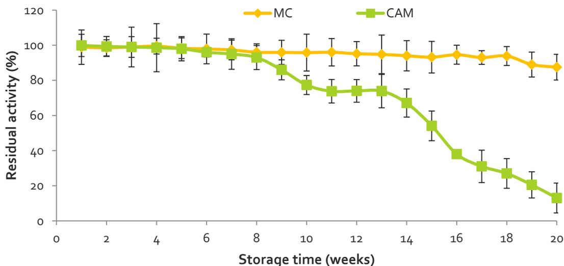
**Figure 4.24: Residual activity in terms of CP biodegradation of MCs and CAMs after several weeks of storage (initial CP 600 mg/L; incubation time 24 h; pH 7; cycles 15)**
