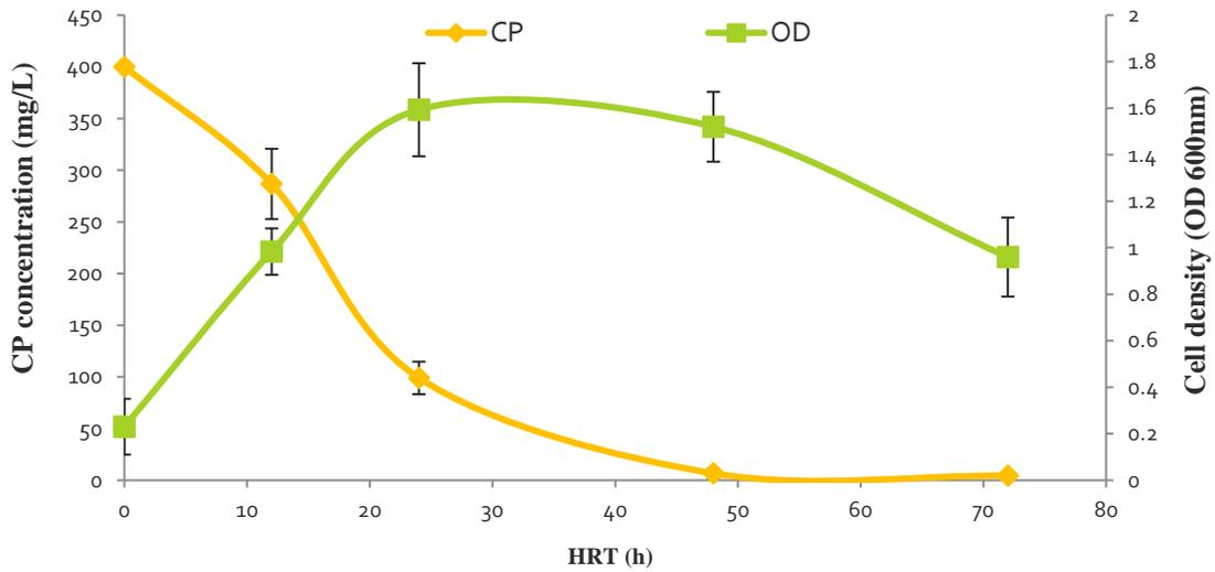
**Figure 4.7: Figure 4.7: Biodegradation of Chlorpyrifos (primary y-axis) and cell density (secondary y-axis) in mineral salt medium supplemented with CP concentrations 400 mg/L; initial inoculum level 10 %; initial pH 7 after variable hydraulic retention time 24, 48, 72h.**
