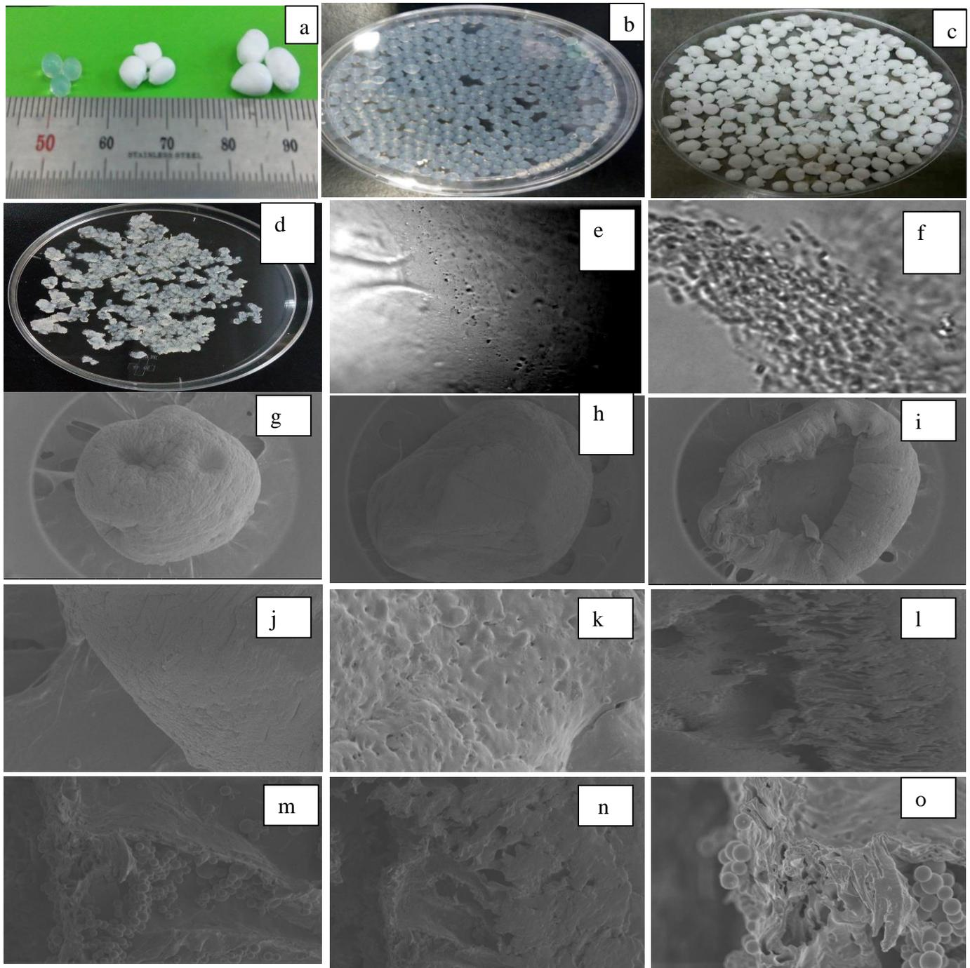
**Figure 4.25: (a, b, c) present CAMs, MCs with single coating, MCs with double membrane coating, photographs of calcium alginate microspheres and macrocapsules (d) disintegrated CAMs (e) microscopic image of MCs (f) microscopic image of bacterial cells**
