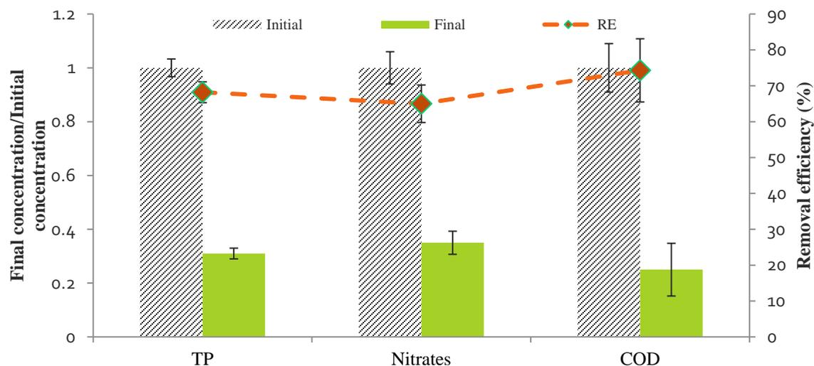
**Figure 4.17: Initial/final concentration and removal efficiency of nitrate (NO<sub>3</sub><sup>-</sup>-N) and phosphate (PO<sub>4</sub><sup>+3</sup>-P) and chemical oxygen demand during biodegradation of CP in WW (CP; 545 mg/L, pH; 7, HRT; 24 h, Glucose; 2 g/L)**
