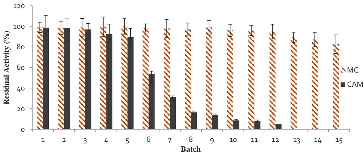
**Figure 4.32: Biodegradation of chlorpyrifos (CP) in real wastewater inoculated with MCs or CAMs for repeated cycles**
