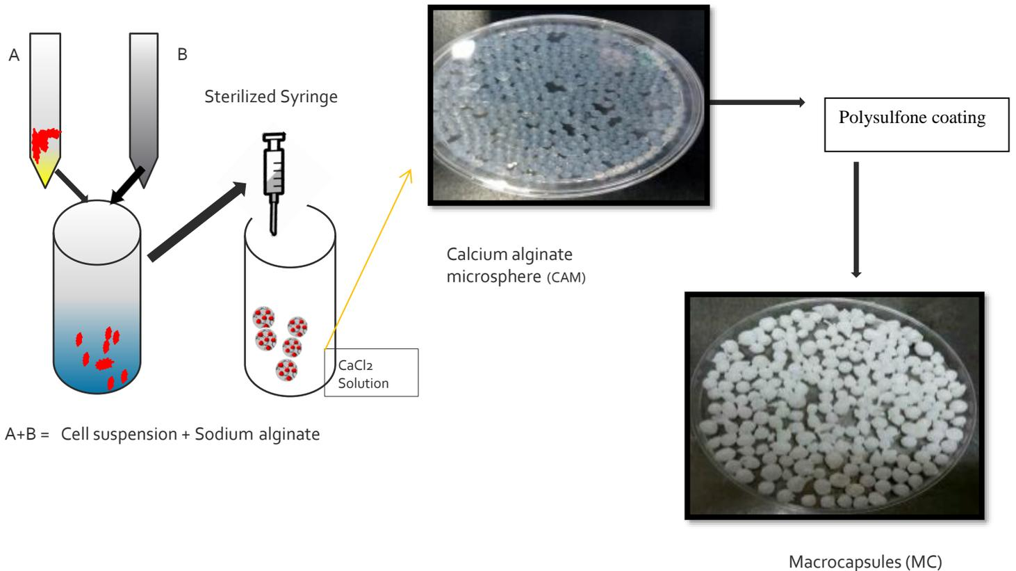
**Figure III a:** Schematic of calcium alginate microspheres (CAMs) and macrocapsules (MCs) preparation process.
