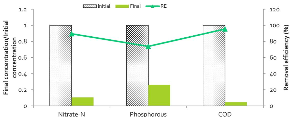
**Figure 4.30: Initial/final concentration and removal efficiency of nitrate-nitrogen ( $\text{NO}_3^-$ —N), phosphate-phosphorous ( $\text{PO}_4^{+3}$ —P) and chemical oxygen demand during biodegradation of CP in MSM inoculated with MCs.**
