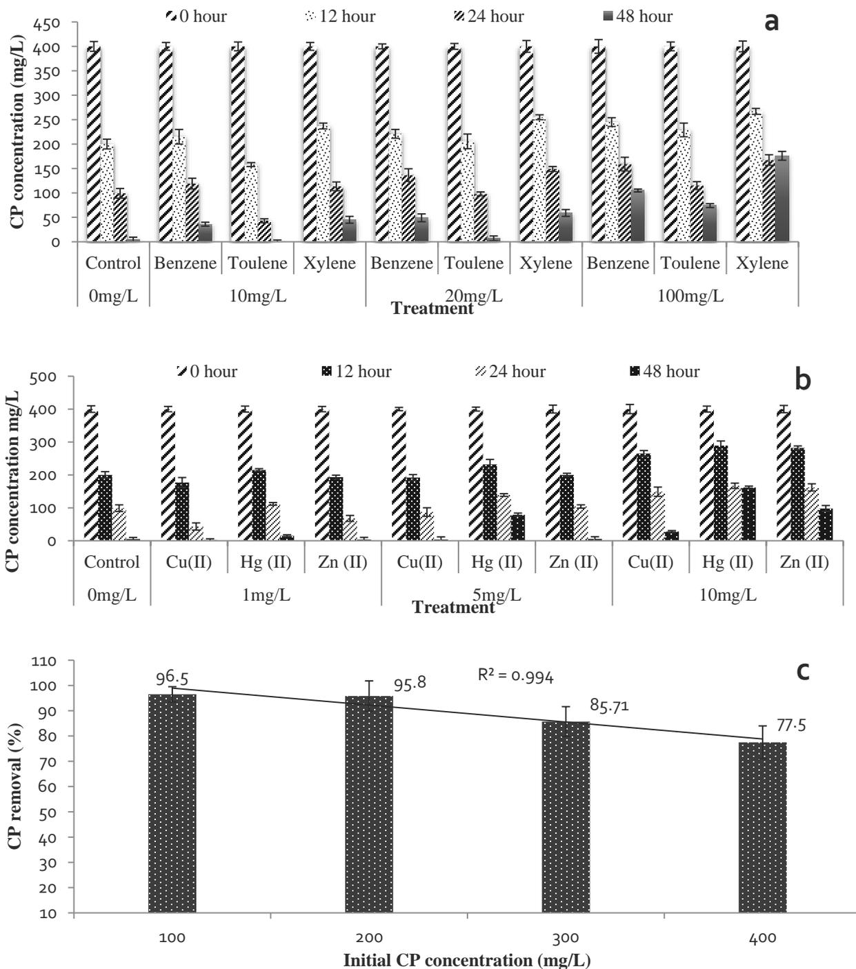
**Figure 4.12: Biodegradation of chlorpyrifos in mineral salt medium at different concentrations of (a) petrochemicals; 10, 20, 100 mg/L (b) trace metals; 1, 5, 10 mg/L (c) in simulated pesticide wastewater at varying CP concentration; 100, 200, 300, 400 mg/L using bacterial consortium**
