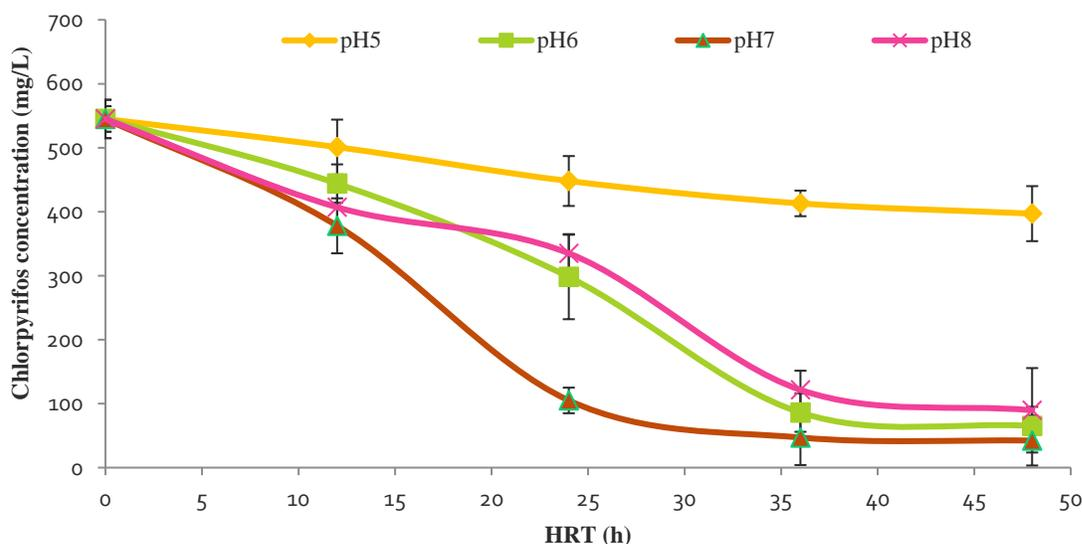
**Figure 4.14: Biodegradation of CP in WW at different pH (5, 6, 7, 8) using bacterial consortium as seeding inoculum (CP; 545 mg/L, HRT; 48h)**
