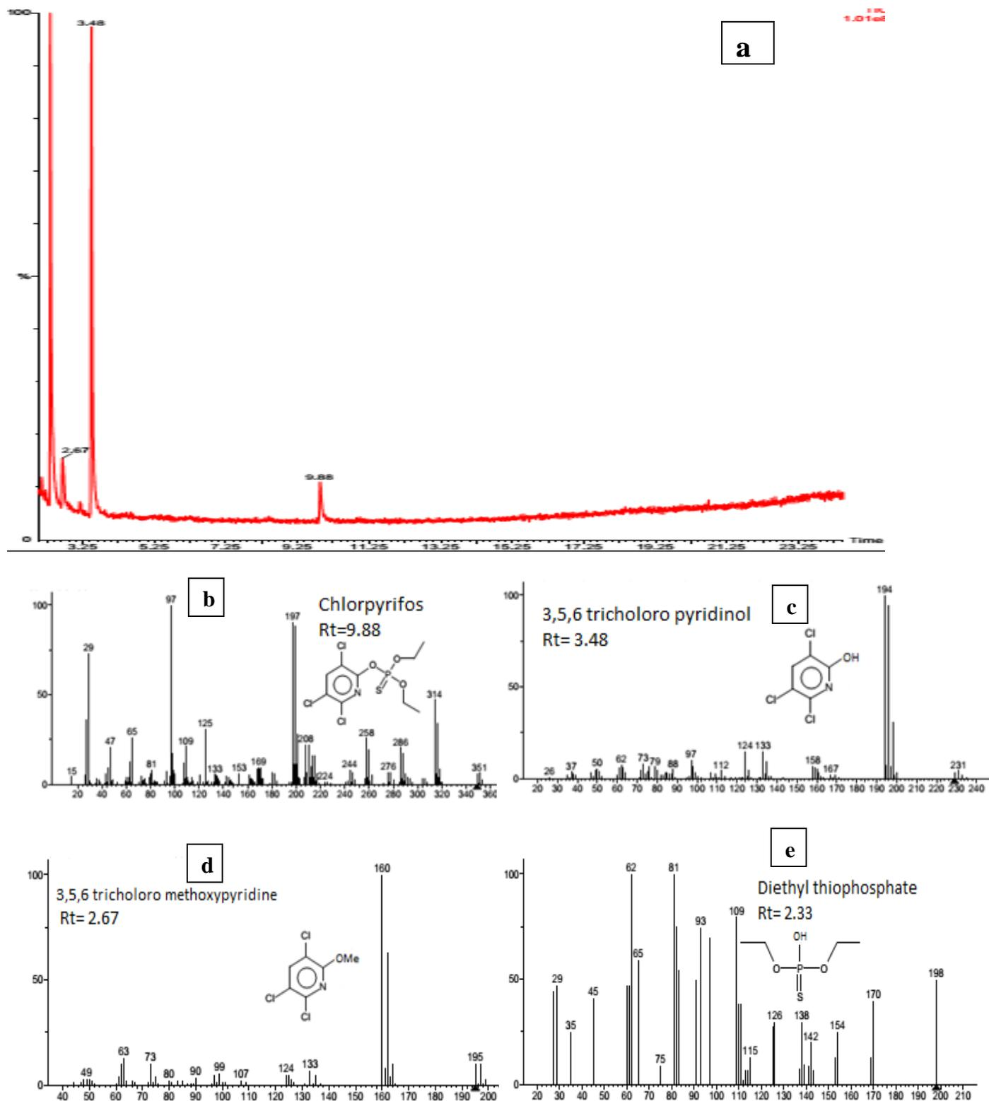
**Figure 4.27:** (a) GCMS chromatogram showing peaks for different metabolites and molecular ion fragmentation pattern of CP (b) and metabolites TCP (c), TMP (d), DETP (e).
