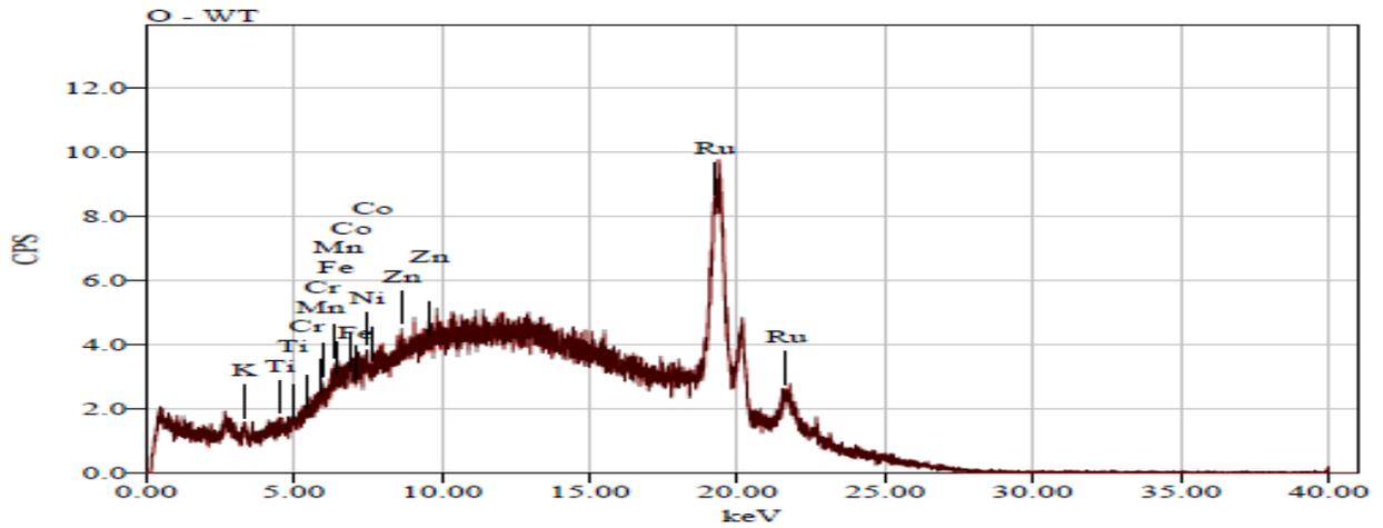
**Figure II b:** XRF pattern of wastewater samples (2) collected from agrochemical industry for various metals (voltage; 30Kv, Current; 1mA, Energy range; 0 - 41KeV, Counting rate; 10565counts/sec).
