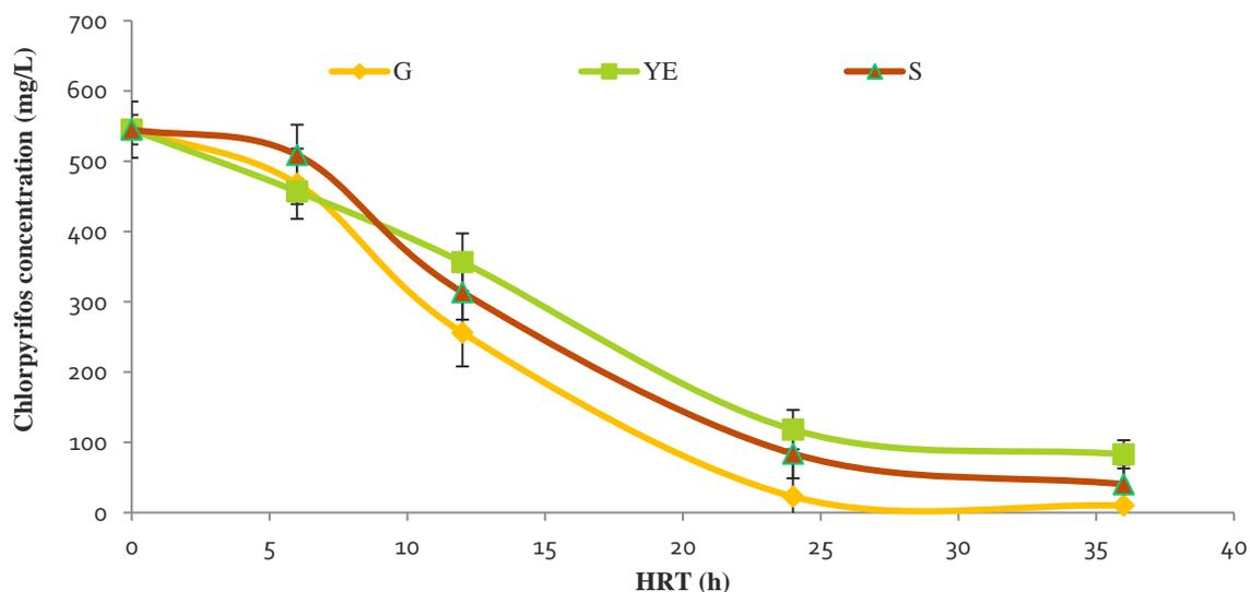
**Figure 4.15: Biodegradation of CP in WW with addition of assimilable carbon substrates i.e. glucose, yeast extract, sucrose (each 2000 mg/L) using bacterial consortium as seeding inoculum. (CP 545 mg/L; pH 7; HRT 36 h)**
