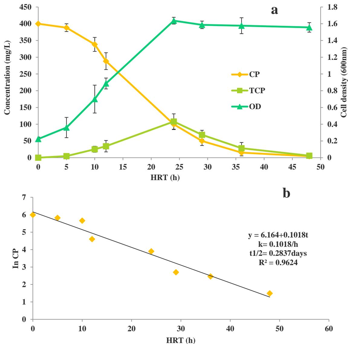
**Figure 4.8: Figure 4.8: Degradation dynamics of CP concentration and TCP formation (mgL<sup>-1</sup>), cell density (600nm) by bacterial consortium (b) relationship of  $\ln(\text{CP})$  and time (Initial CP concentration: 400 mg/L, initial pH: 7, HRT;48 h).**
