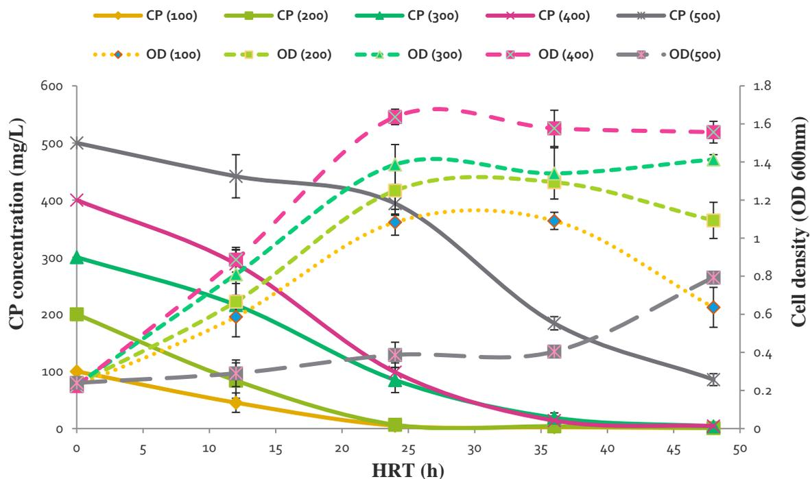
**Figure 4.6: Figure 4.6: Biodegradation of Chlorpyrifos (primary y-axis) and cell density (secondary y-axis) in mineral salt medium supplemented with various CP concentrations from 100 to 500 mg/L of mineral salt medium (initial inoculum level 10%; initial pH 7; HRT 48h)**
