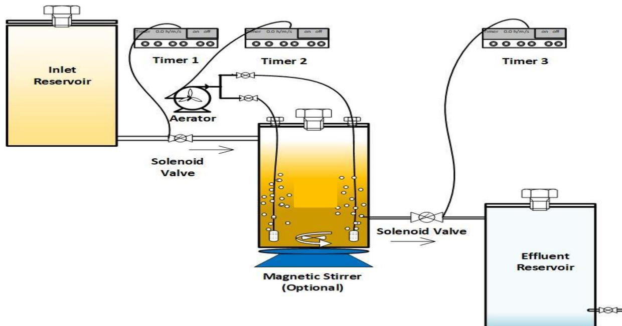
**Figure 3.1: Schematic layout of laboratory scale batch reactor (1) inlet reservoir (2) air tank (3) effluent reservoir**
