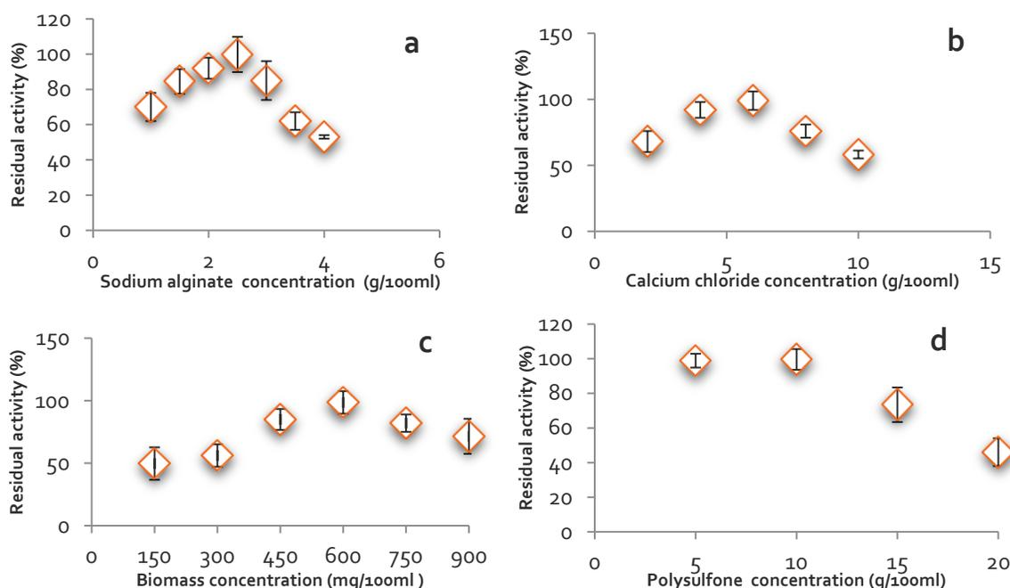
**Figure 4.20: Effect of different concentrations of (a) sodium alginate (b) calcium chloride (c) biomass concentration (d) polysulfone on residual activity of MCs**
