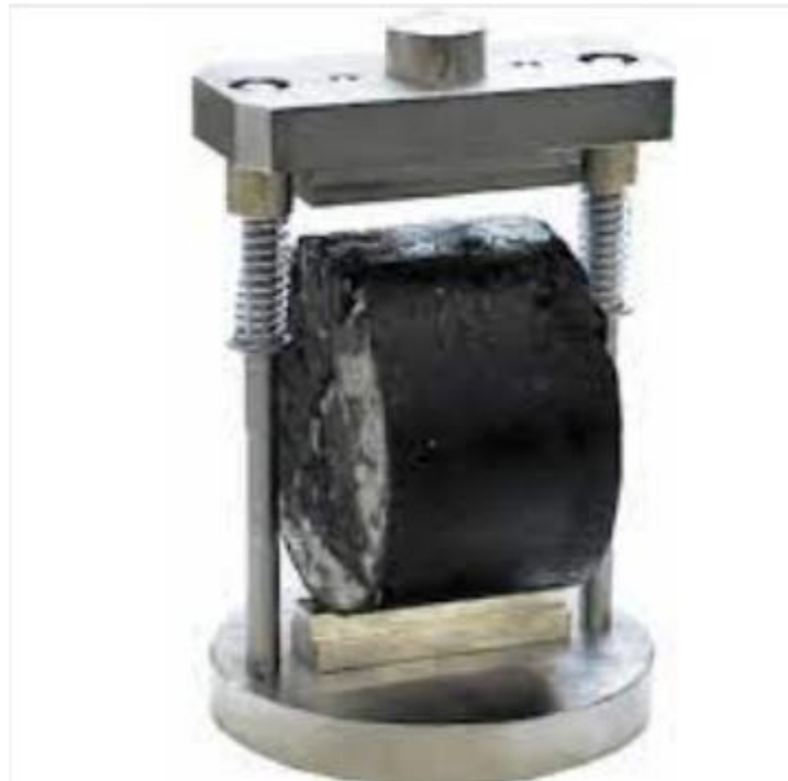
Figure 3.6.2 (b) Block placed in Marshall test machine.
