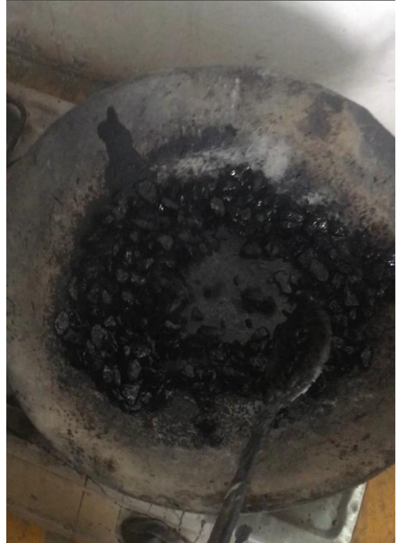
Figure 3.3.3 (a) Group member Faisal giving blows to the sample and (b) Aggregates being heated along with the bitumen.
