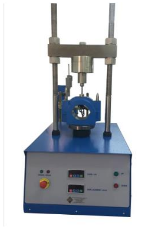
Figure 4.5 (a) Machine showing Marshall Stability Test machine.
