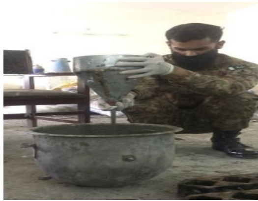
Figure 3.4.1 (a) Flow cone showing how the flow grout test is performed and (b) Group leader Mohammad performing the flow cone test.
