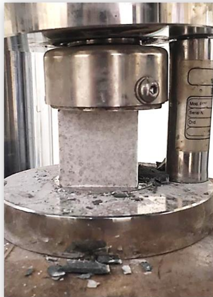
Figure 2.3.2 Cement grout cube undergoing Compressive Strength Test
