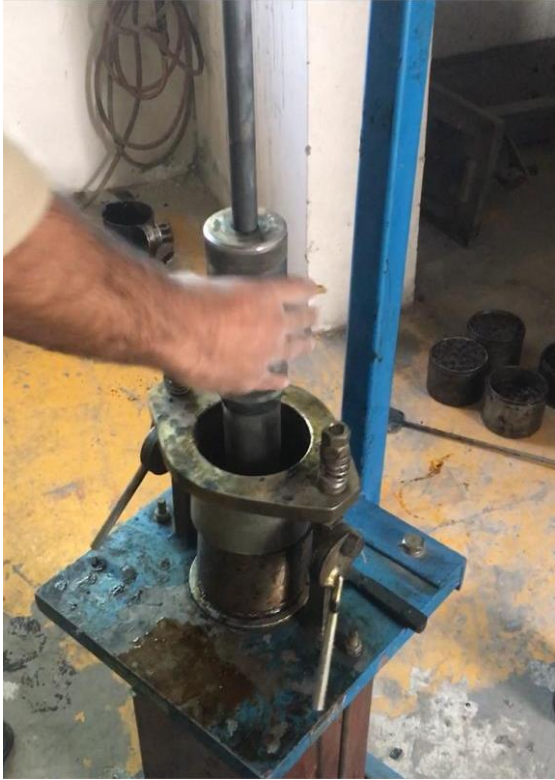
Figure 3.3.3 (a) Group member Faisal giving blows to the sample and (b) Aggregates being heated along with the bitumen.
