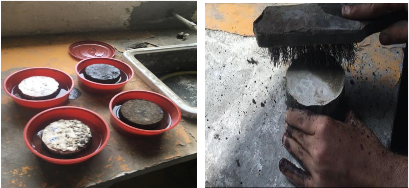
Figure 3.6.1 (a) Samples submerged in diesel and (b) Sample being subjected to abrasion by steel brush by group member Abubakr.
