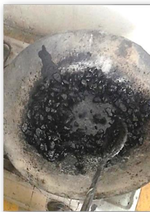
Figure 2.3.1 Mixing of open-graded asphalt specimens
