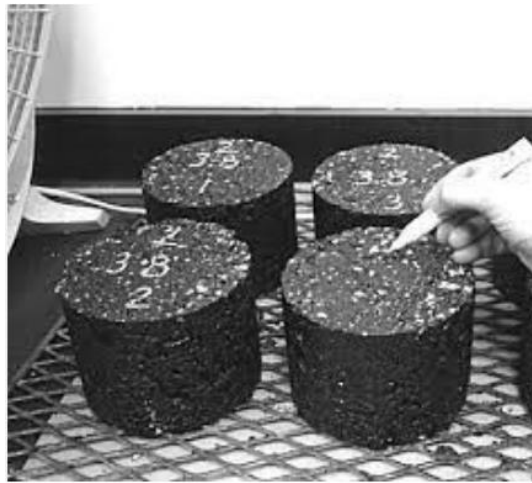
Figure 4.4 (a) Marking of specimens (HMA) before submerging them into diesel.
