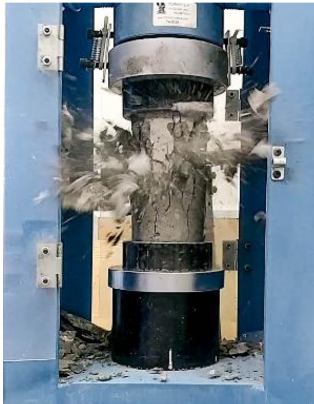
Figure 4.2 Block undergoing compressive strength test.
