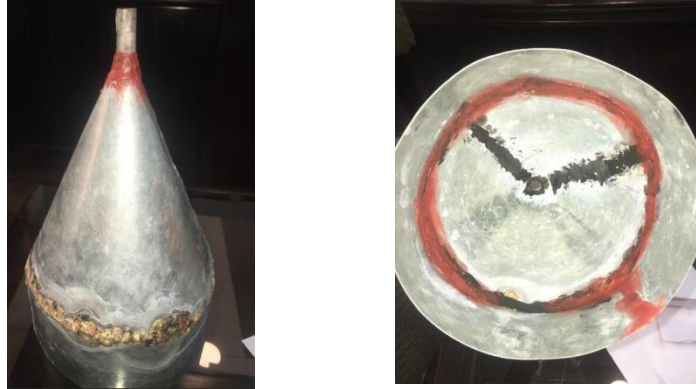
Figure 3.1.3 Welded Flow Cones – Max V = 1725ml.
