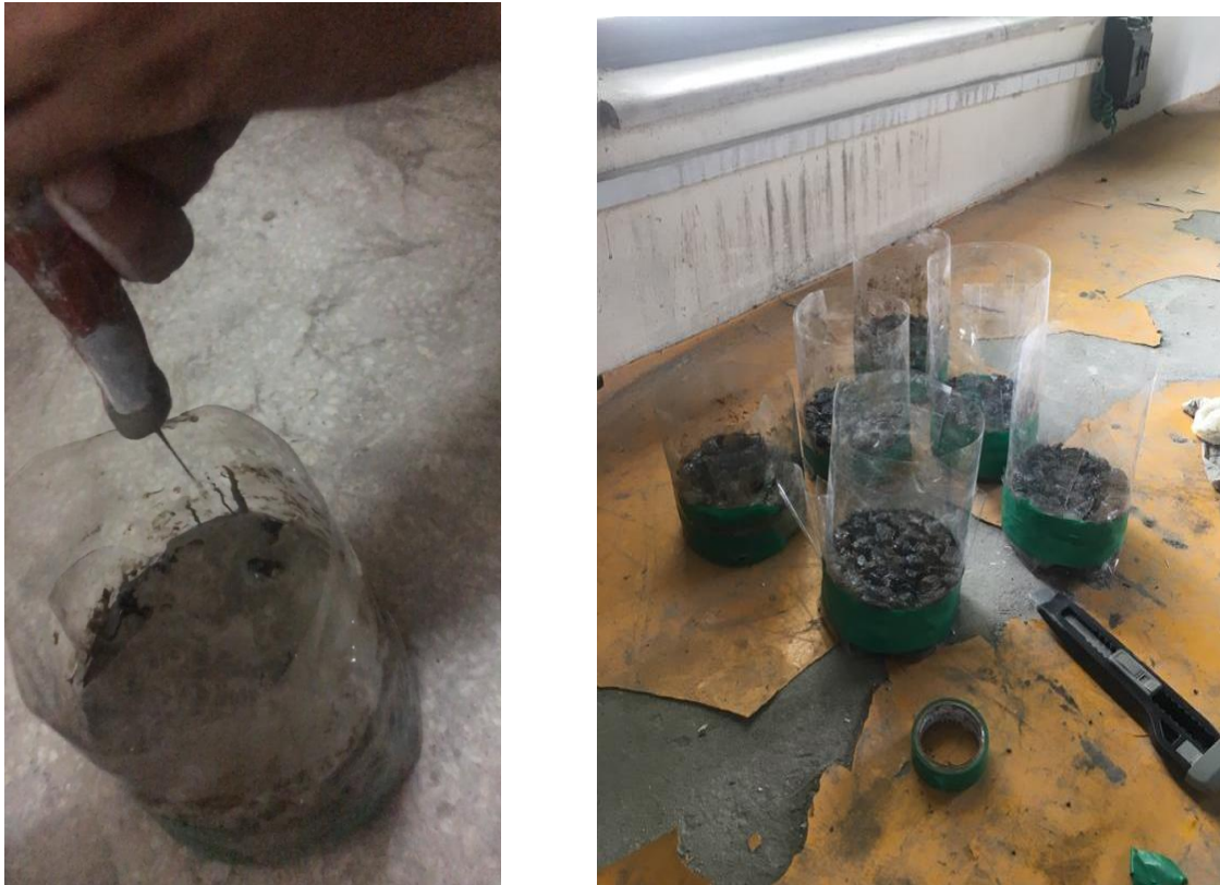
Figure 3.3.4 (a) Grouts being poured into the open-graded specimen and (b) open-graded specimens wrapped in a talic sheet.
