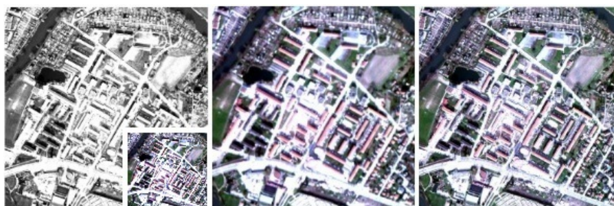
Figure 4.1: Sample image used for Case 01 (From left to right HR PAN, LR MS, upsampled LR MS and HR MS image).
