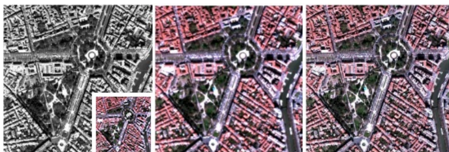
Figure 4.3: Sample image used for testing in Case 02 (From left to right HR PAN, LR MS, upsampled LR MS and HR MS image).
