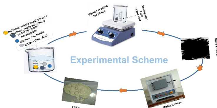
Figure 7: Synthesis of LSTN perovskite
