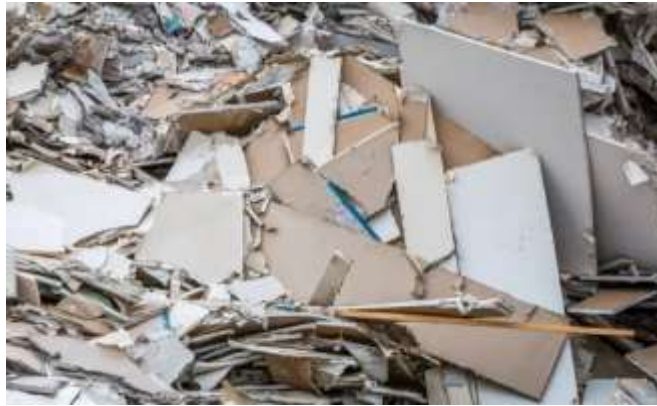
Figure 3 Gypsum waste (Demolition) Richard Thomas Lerman, 2023
