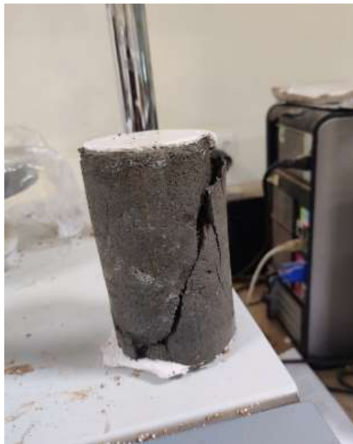
Figure 20 Sample failed in shear
