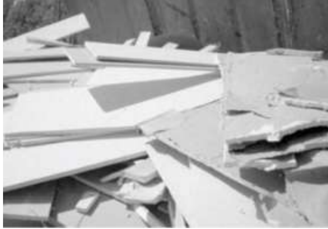
Figure 2 Gypsum waste (New construction) Richard Thomas Lerman, 2023
