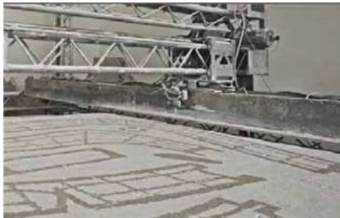
Figure 24: Binder jet 3D printing [24]
