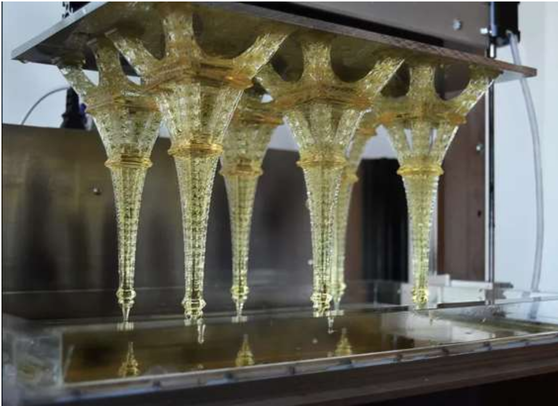
Figure 16: Digital Light Processing 3D printer [20]
