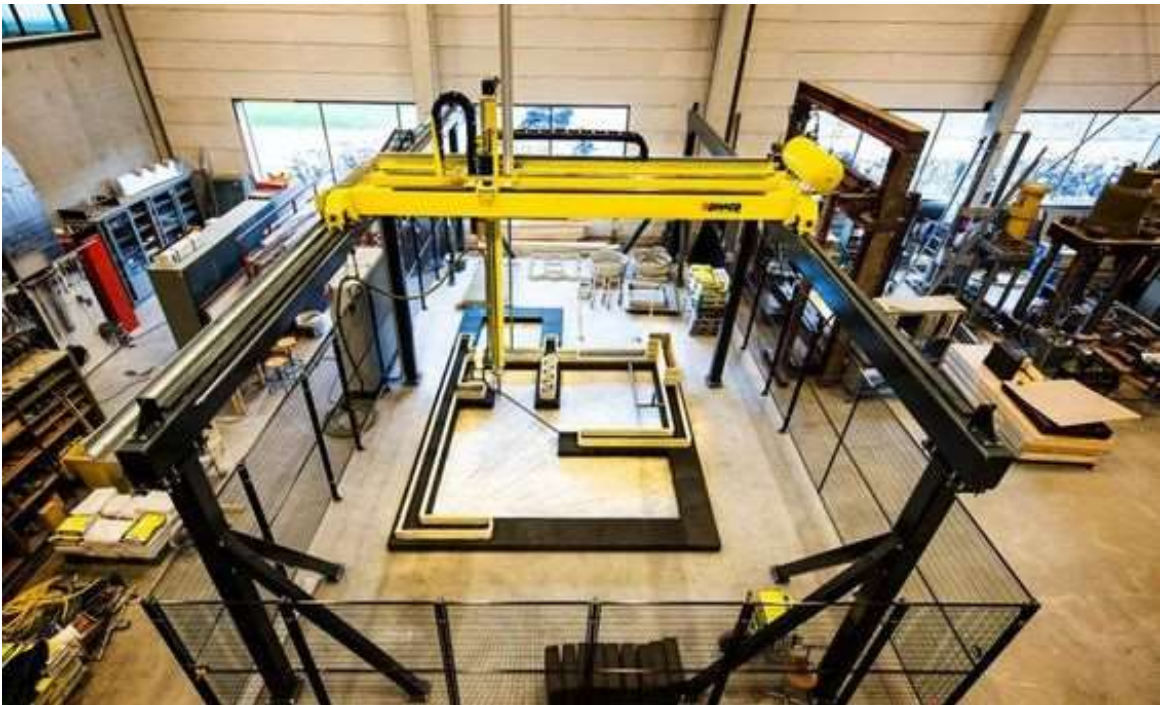
Figure 21: Concrete 3D printer [22]
