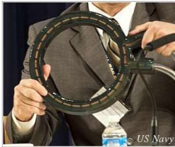
Figure 4: 3D printed undersea wireless charger
