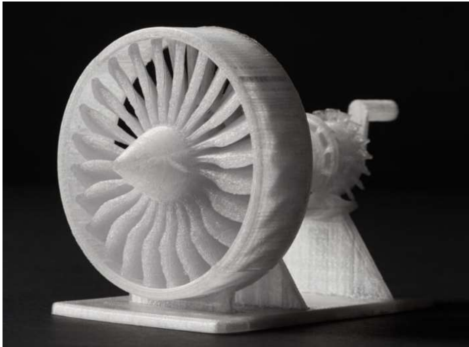
Figure 12: 3D printed prototype Fused deposition method [17]
