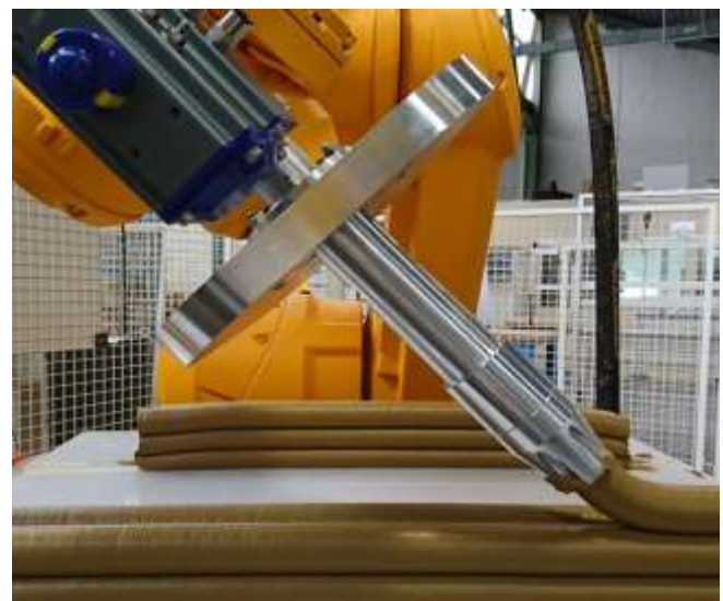
Figure 23: Actual layered extrusion 3D printer [23]
