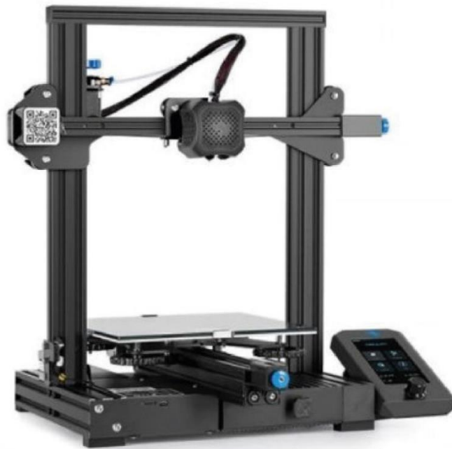
Figure 3.2 ENDER 3 V2 FDM PRINTER
