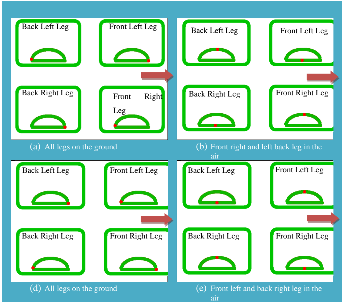
Figure 6.6 Gait generation in processing software
