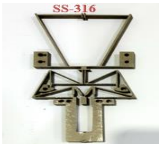
Figure 4-8: Manufactured two stage amplifier
