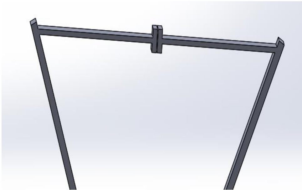
Figure 2-11: Schematic of normally close microgripper design
