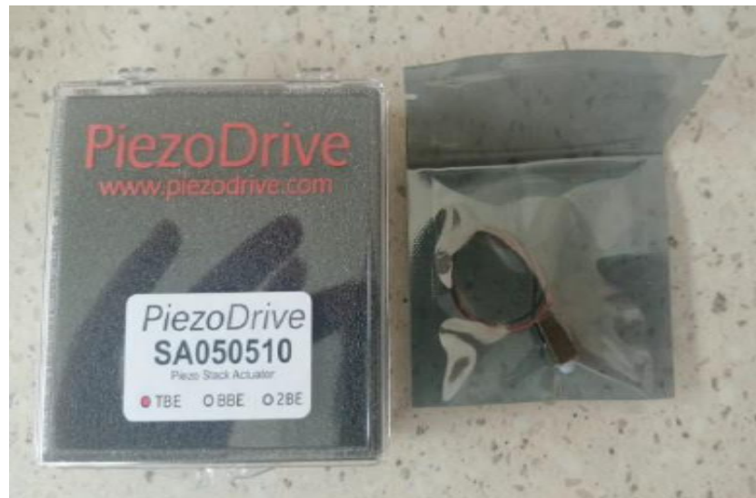
Figure 2-13: Selected Piezoelectric Actuator
