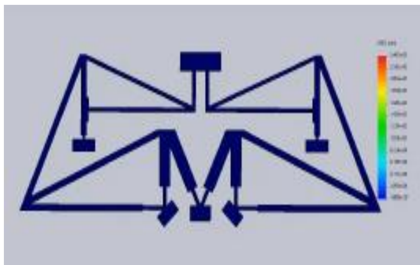
Figure 3-5: ANSYS analysis for stage II amplification.
