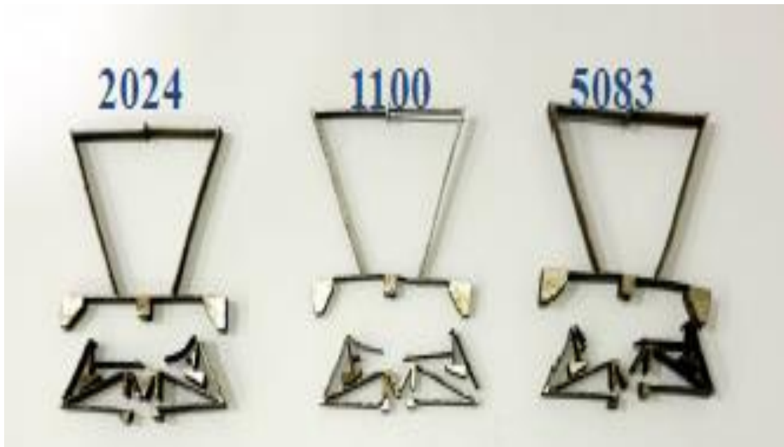
Figure 4-7: Structures of raptured manufactured designs.
