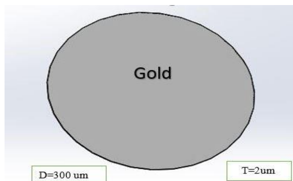
Figure 2.6: A schematic diagram of micromirror.
