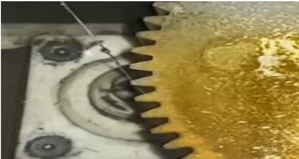
Figure 31: Gear cutting operation on AISI 1045 medium carbon steel
