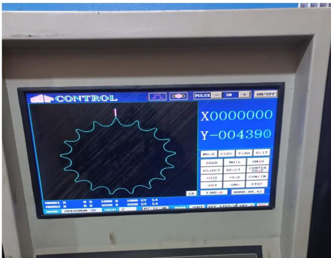
Figure 29: H.F. control system working on teeth's profile
