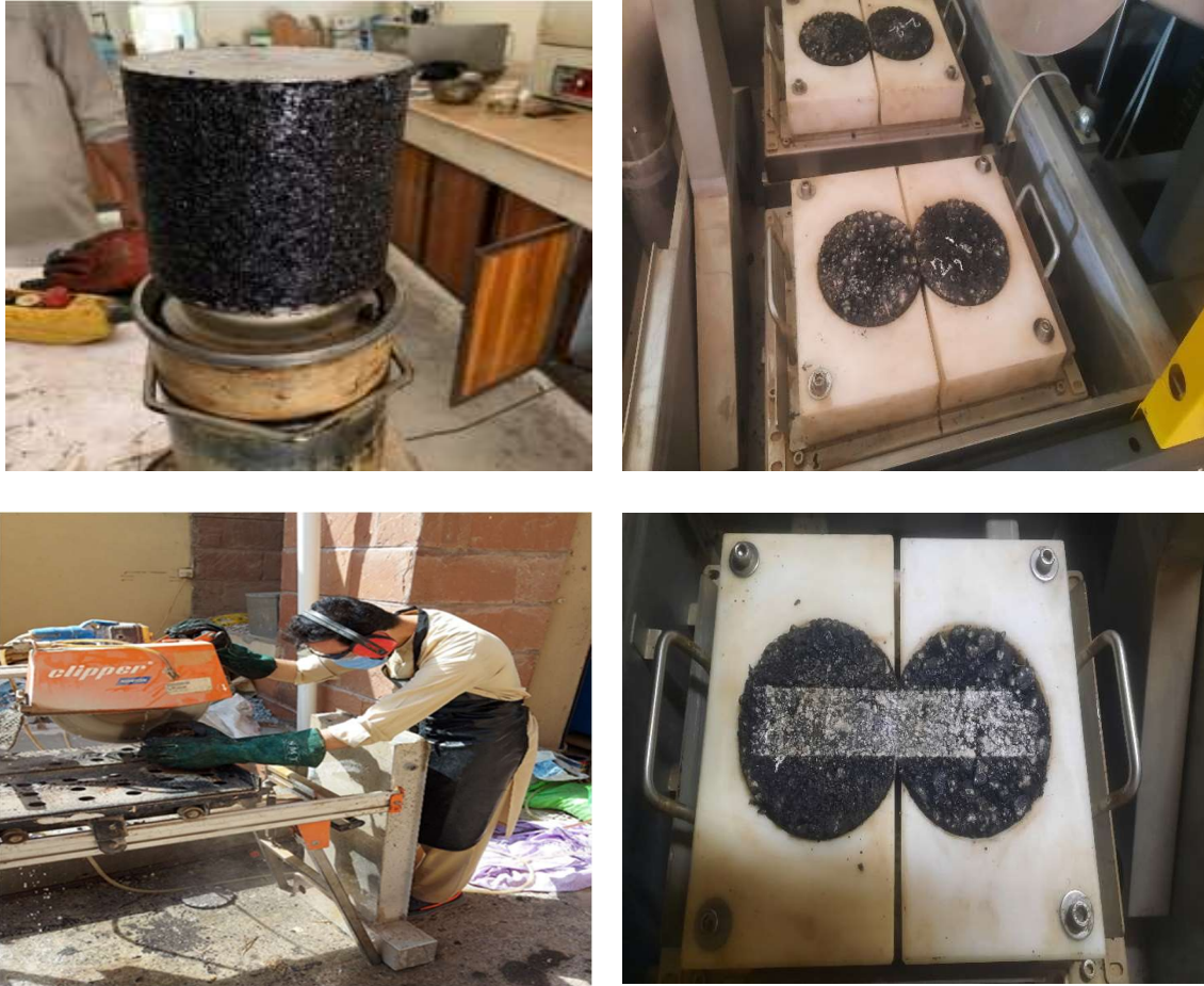
Figure 3. 17: Rutting Samples Preparation and Testing
