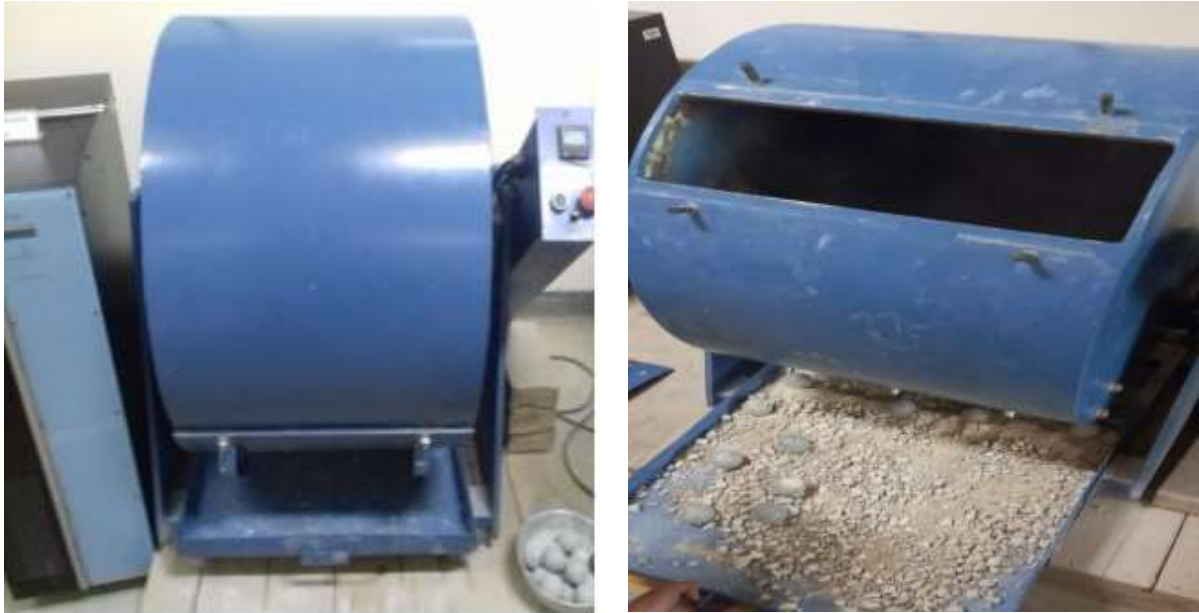
Figure 3. 6: Loss Angeles Abrasion Machine & Testing
