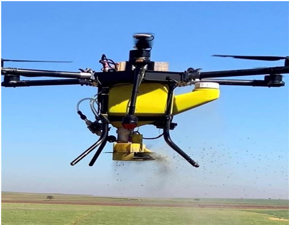
Figure 1.4:Multi Rotor Drone-Borne Aerial Fertilizer Spreader you can see in figure (1.4).
