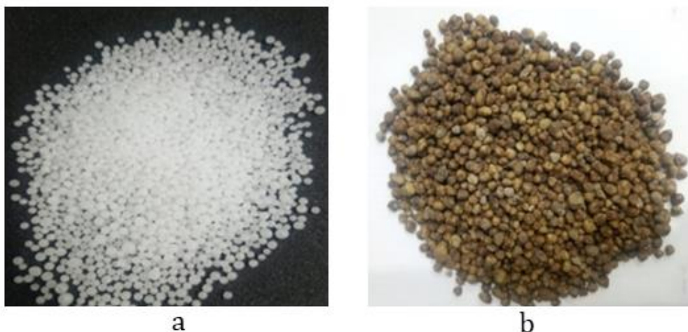
Figure 4.1 (a) Urea Fertilizer (b) DAP Fertilizer particle diameter was 2mm, the bulk density was taken 2000 kg/m 3 . Table 4.1 show the diameter were bulk density of urea fertilizer.
