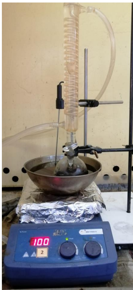
Figure 14: rGO synthesis assembly
