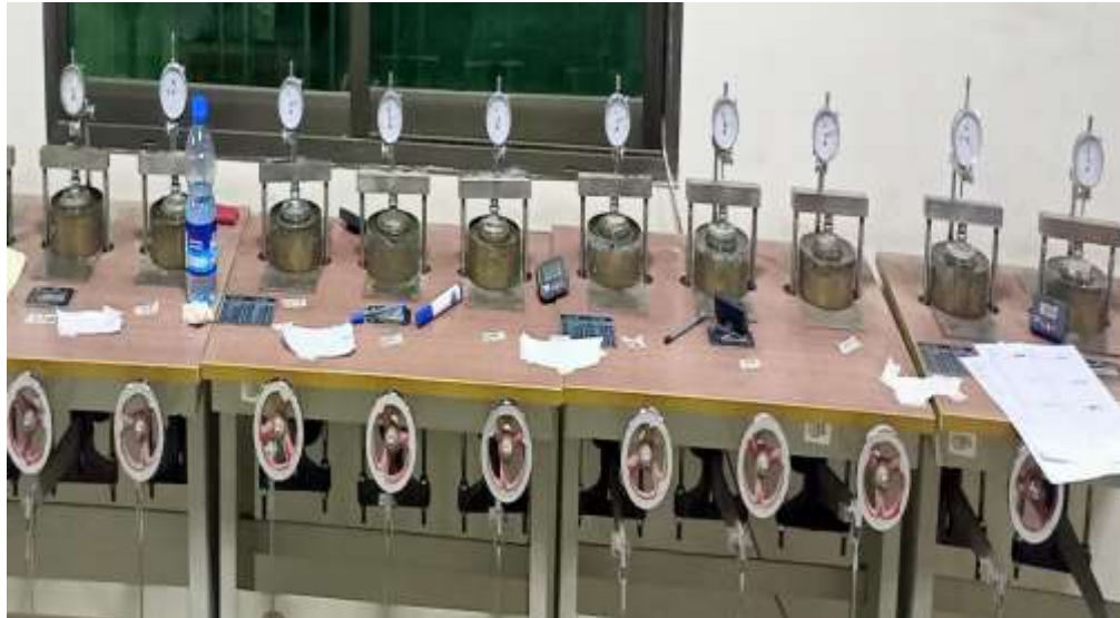
Figure 23: Swell Percent Test Performed on the Soil Mixed with CCR:WSA Binder
