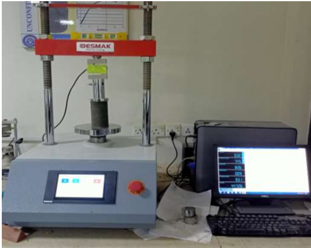
Figure 20: Unconfined Compression Test Performed in the Laboratory
