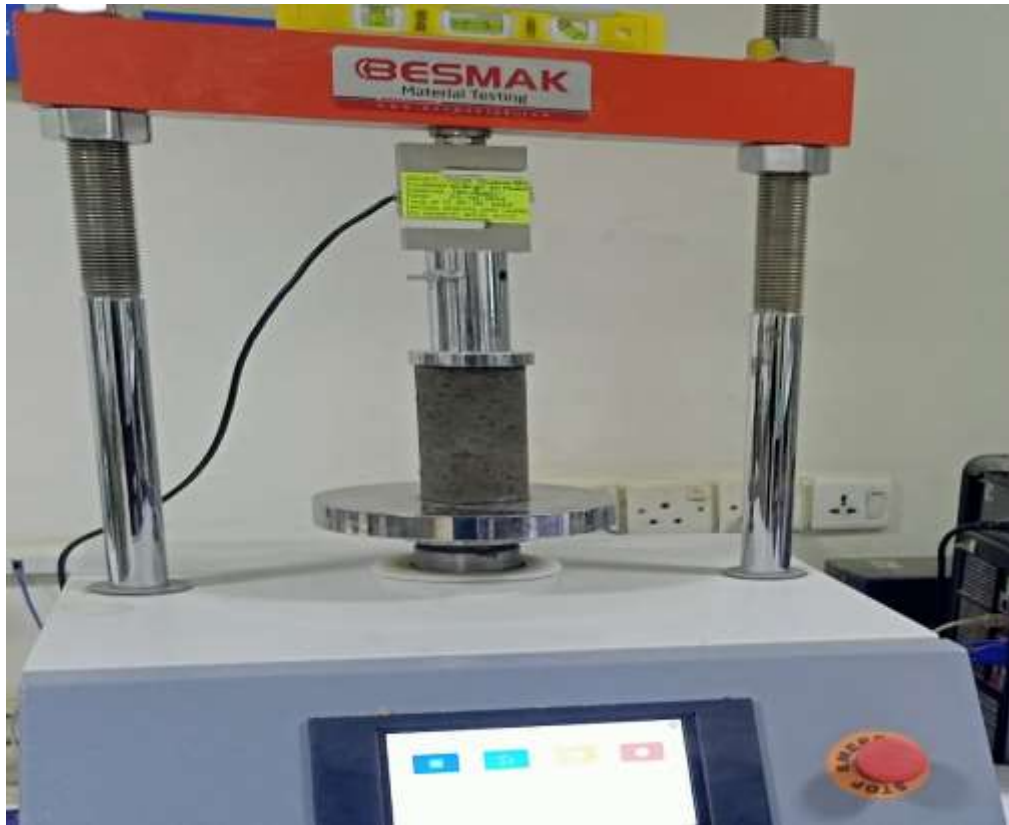
Figure 24: UCS Test Carried out on the Soil Stabilized with CCR:WSA Binder
