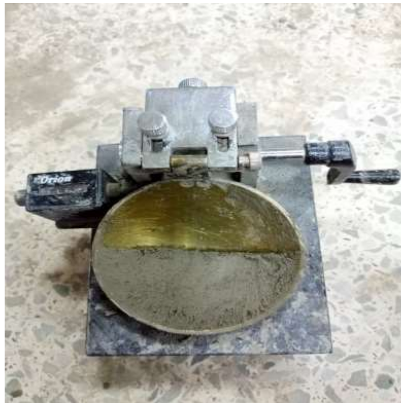
Figure 16: Liquid Limit Test by Casagrande Apparatus
