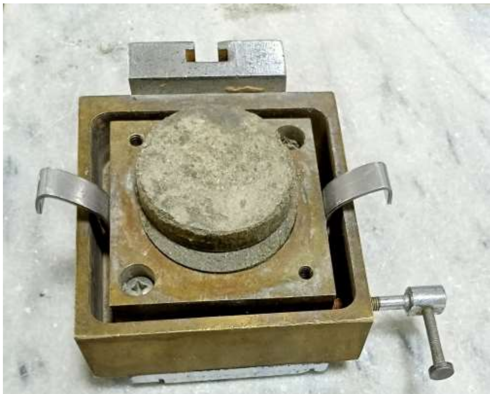
Figure 25: DST Test Carried out on the Soil Stabilized with CCR:WSA Binder
