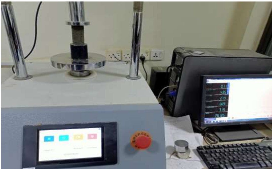
Figure 22: UCS Test Performed on the Soil Mixed with WSA
