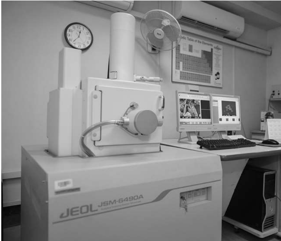
Figure 28: SEM & EDS Test performed on JEOL JSM-6490A
