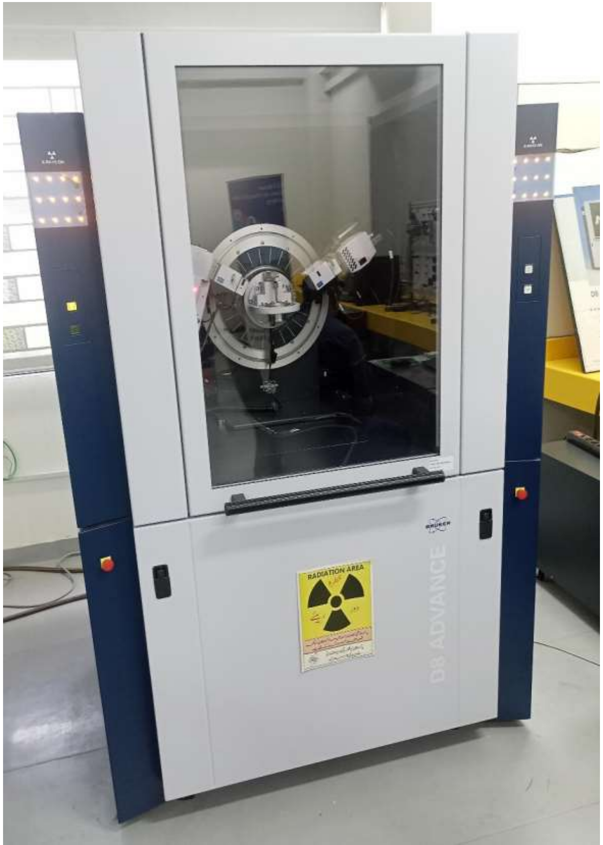
Figure 27: XRD Test performed on Bruker D8 Advance Diffractometer
