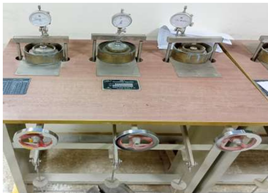
Figure 19: Swelling Pressure Test carried out in Laboratory
