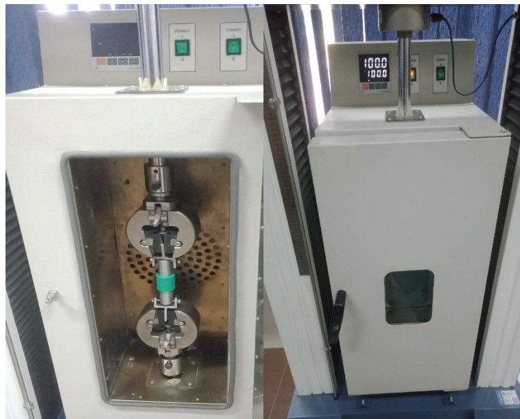
Figure 3.10: Adhesive joint during testing at 100 degrees temperature
