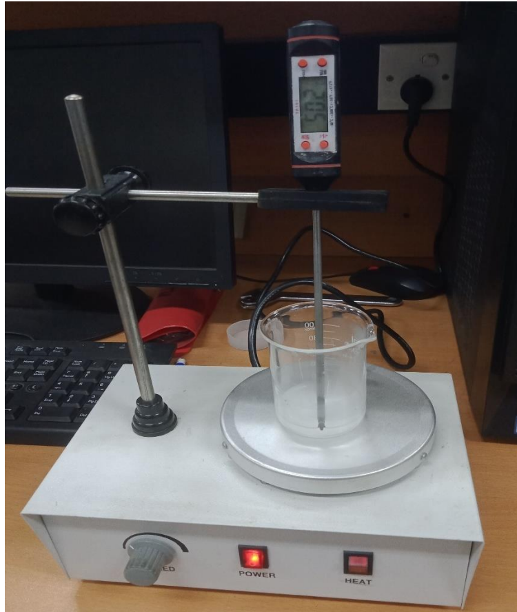
Figure 3.6: Stirring of epoxy adhesive on magnet stirrer.
