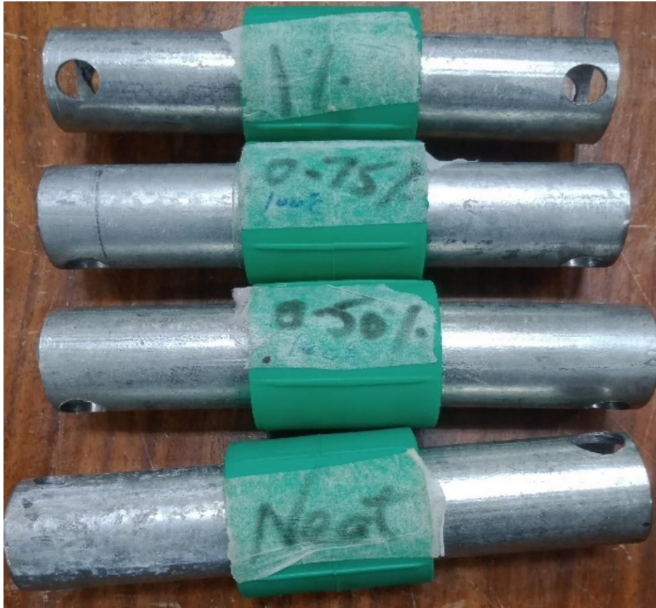
Figure 3.7 Adhesive joints of steel and PPR pipes at different cork concentrations
