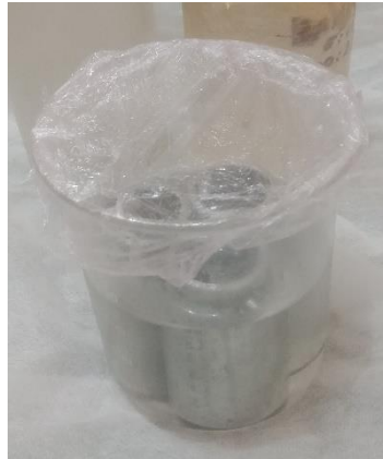
Figure 3.4: Cleaning steel surface with acetone
