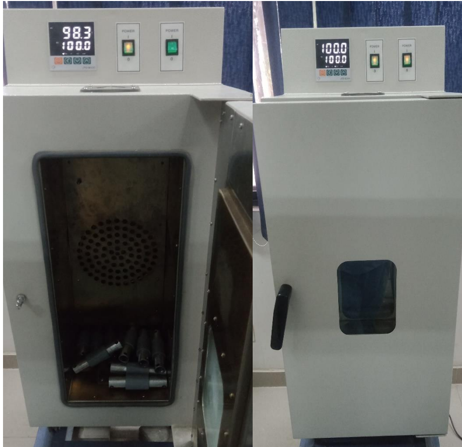
Figure 3.8: Curing of joints in oven at 100 degrees temperature
