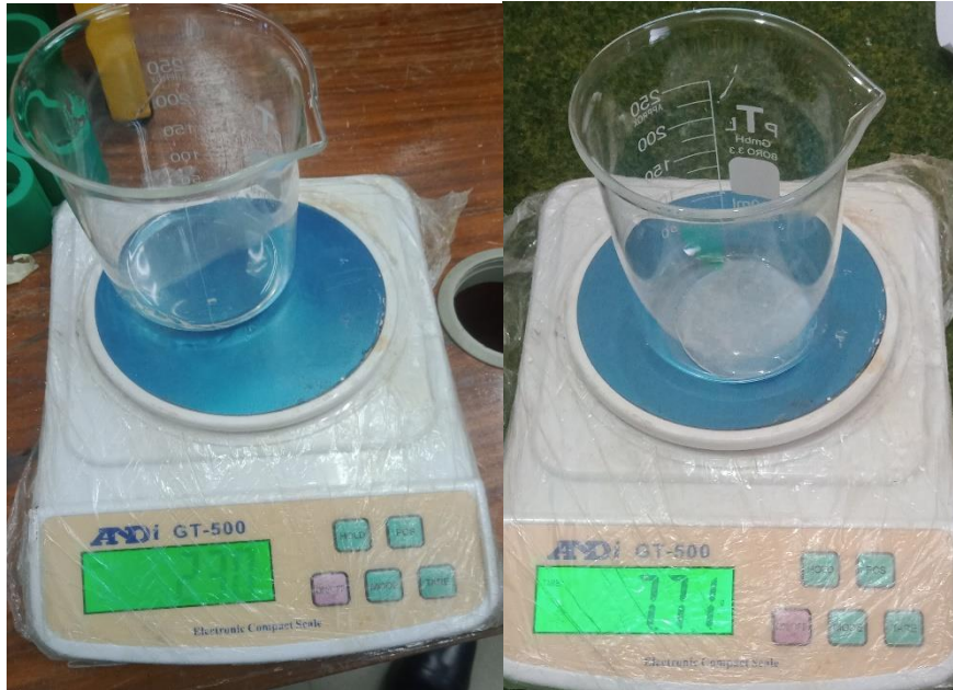
Figure 3.5: Weight measurement for epoxy and hardener
