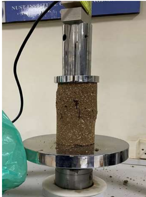
Figure 3.6 Unconfined Compression Tests for EPS mixed clayey soil
