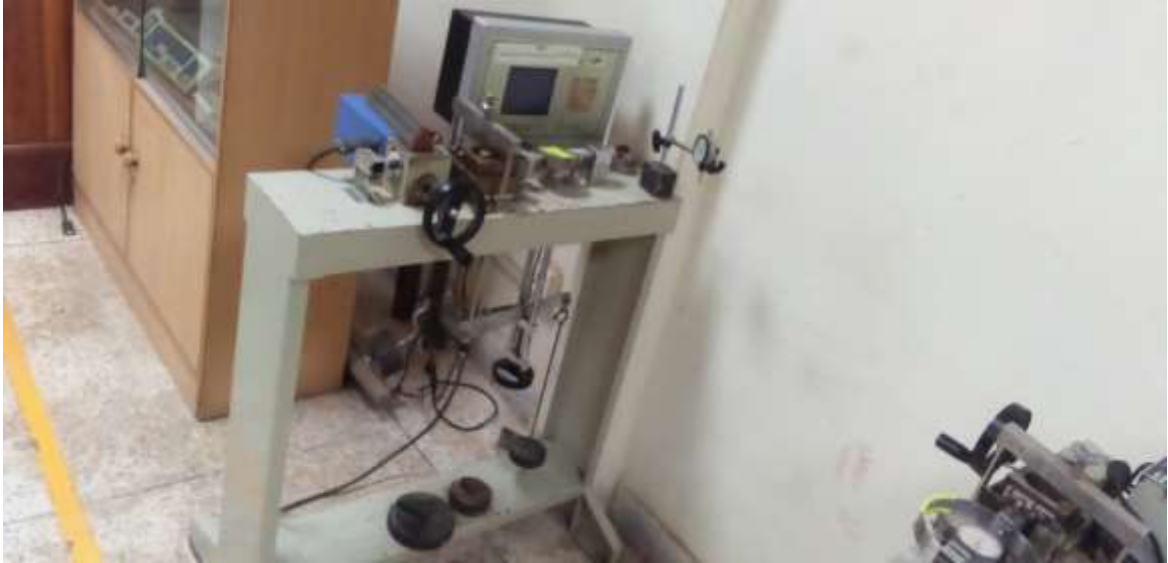
Figure 3.7 Direct Shear Apparatus used in the present study
