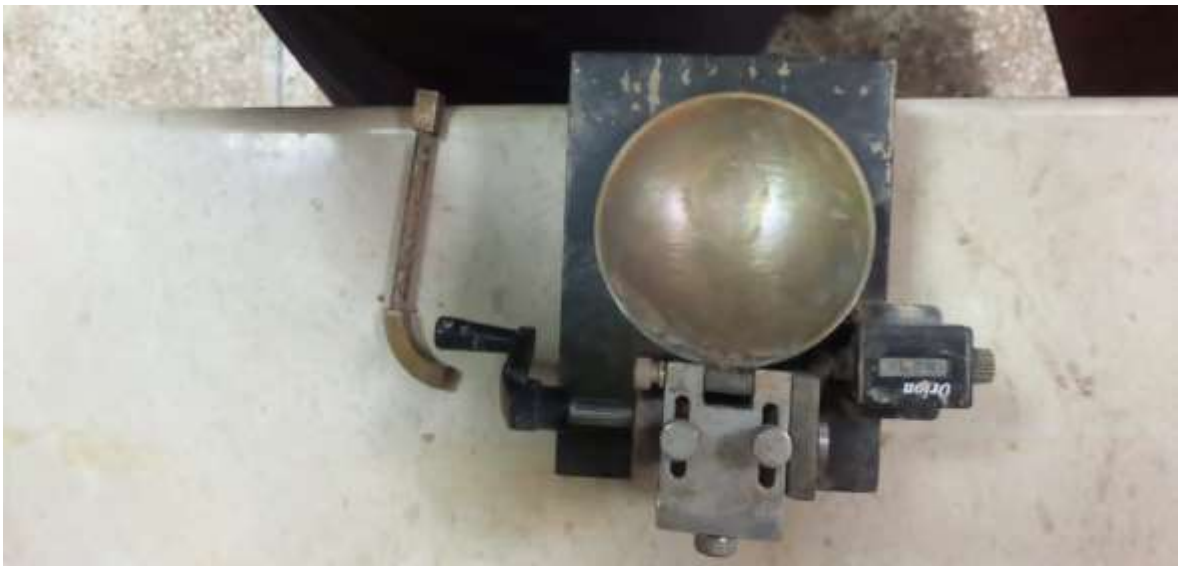
Figure 3.8 Casagrande Test Apparatus used in the present study
