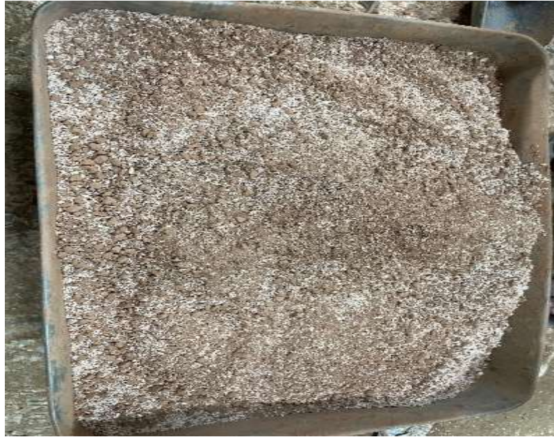
Figure 3.4 Preparation of EPS-clay sample (Medium Plastic Soil)
