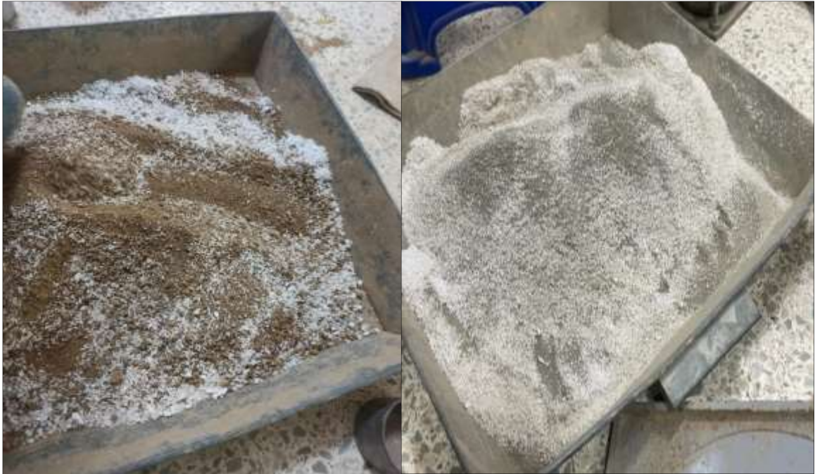
Figure 3.5 Preparation of samples for proctor test (High Plastic and Low Plastic Soils)
