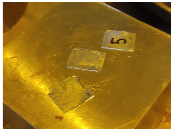
Figure 2-10: Electrodes after compressing
