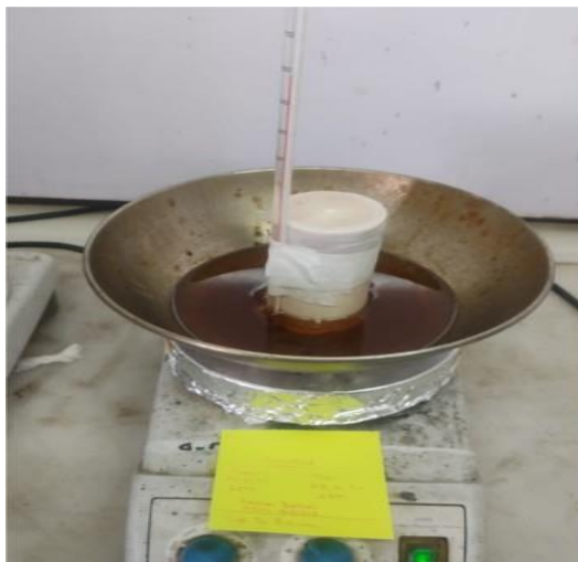
Figure 2-2: Mixing of chemicals by Magnetic Stirring
