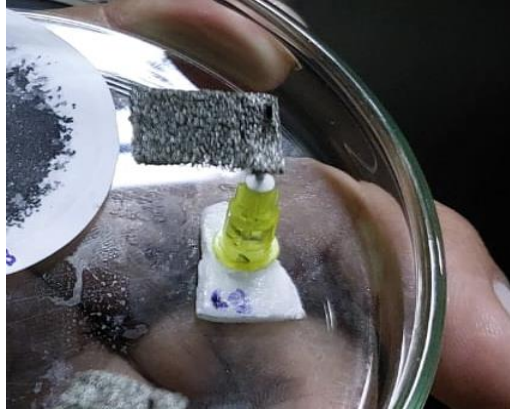
Figure 2-9: Dispersion of material over Nickel foam
