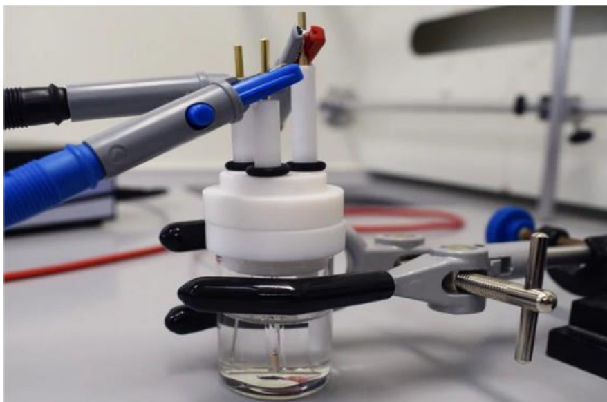
Figure 2-15: Three Electrode cell as used in cyclic voltammetry with an Ossila Potentiostat
