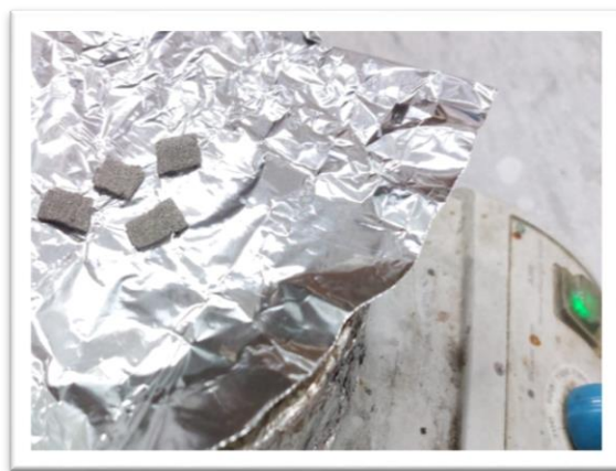
Figure 2-8: Drying of Nickle foam
