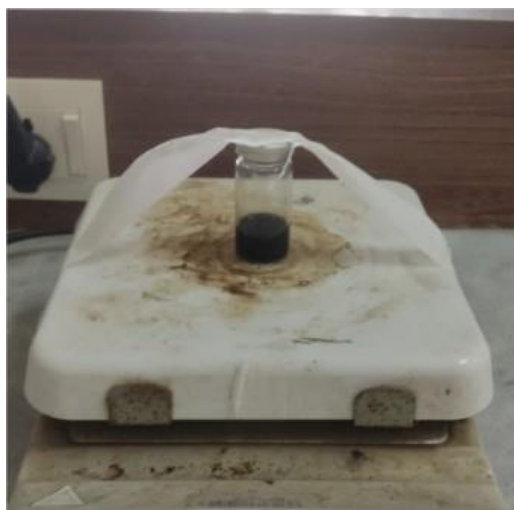
Figure 2-5: Stirring at Hot Plate of MXene
