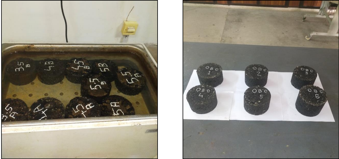
Figure 3.23. Indirect tensile strength and tensile strength ratio test
