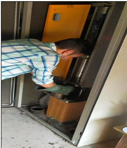
Figure 3.21. Preparation of Marshall samples and testing
