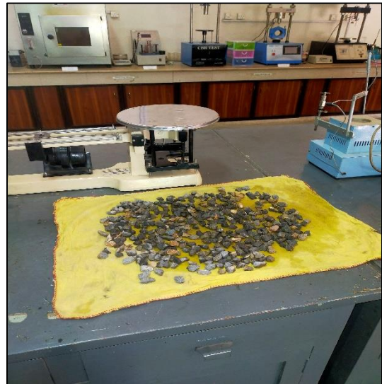
Figure 3.8. Specific gravity and water absorption test (Coarse aggregate)
