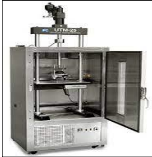
Figure 2.4. ITS test assembly (www.innopave.com)
