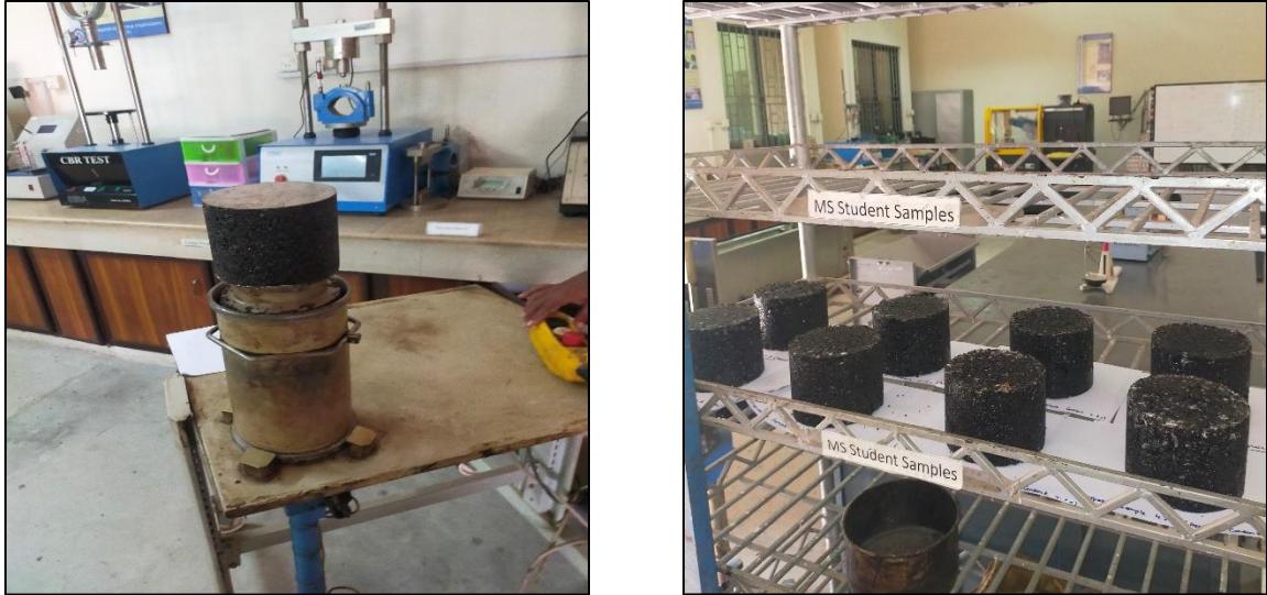
Figure 3.19. Specimens preparation for Superpave asphaltic concrete mixture
