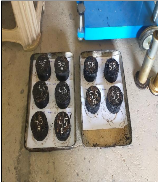
Figure 3.20. Marshall asphalt mix samples and Marshall stability machine
