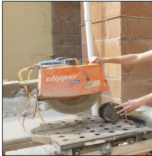
Figure 3.22. Core cutting of compacted asphalt sample
