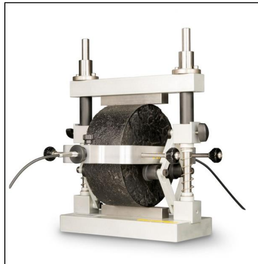
Figure 2.3. Resilient modulus test assembly (www.jetmaterials.com)
