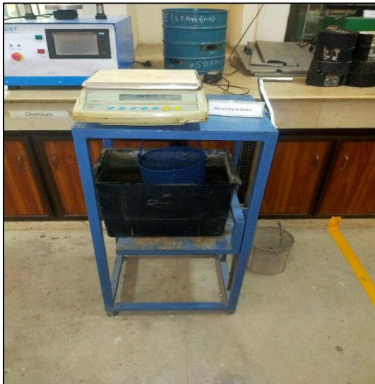
Figure 3.8. Specific gravity and water absorption test (Coarse aggregate)
