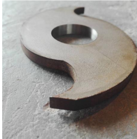
Figure 11 Rotary Blade Manufactured through EDM
