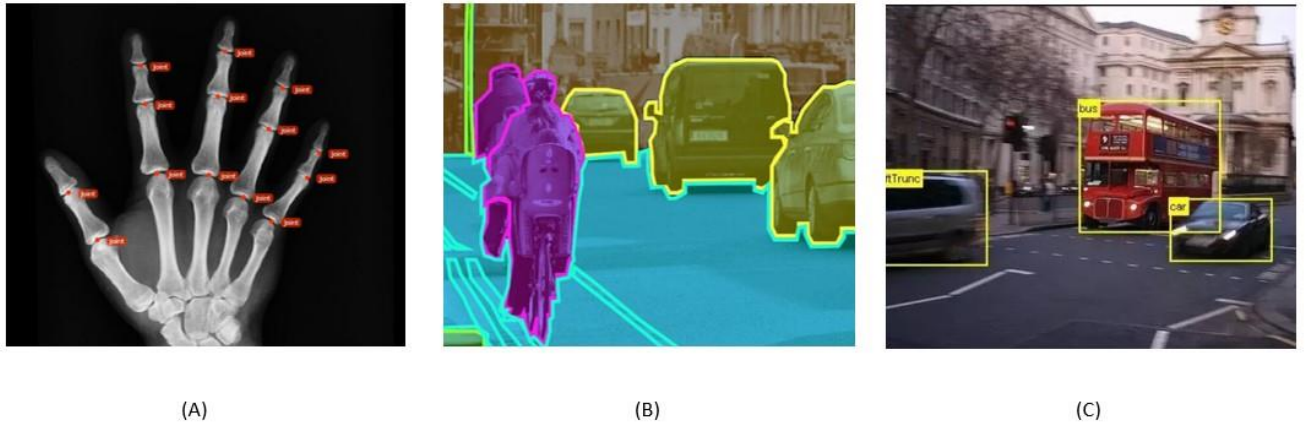
Figure 17 Examples of Image Labelling (A) shows Key Points labeling, (B) represents semantic Segmentation and (C) represents the bounding box labelling
