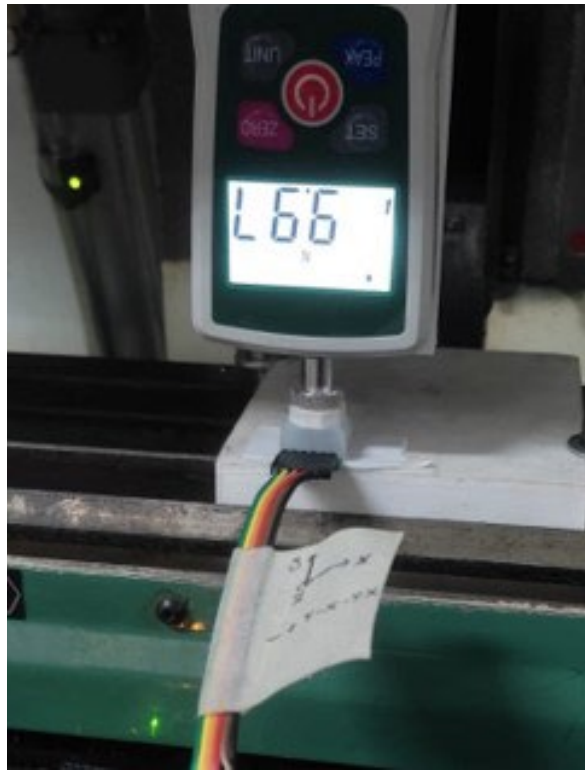
Figure 4.7 Force application on the sensor face using the force gauge probe
