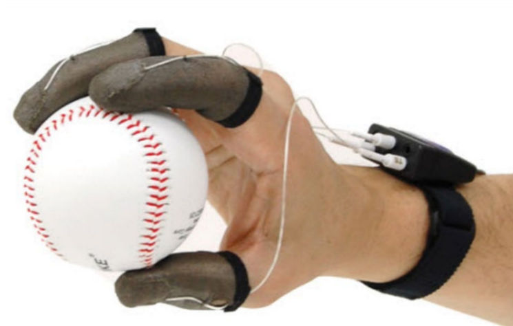
Figure 1.3 A wearable tactile sensor for object grasping feedback [17]
