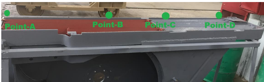
Figure 4.1: Points of observation of air flow velocity
