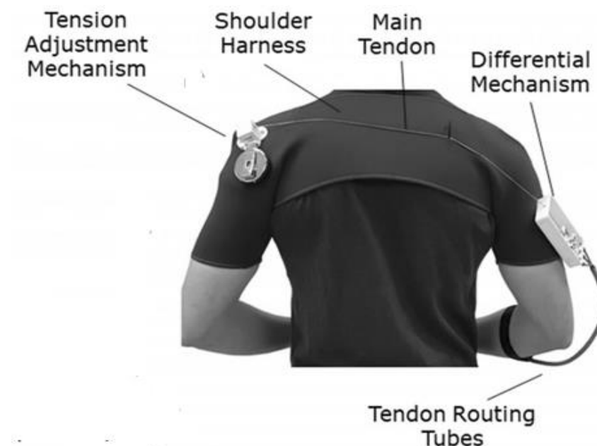
Figure 3.1 Annotated presentation of the body-powered device[87]
