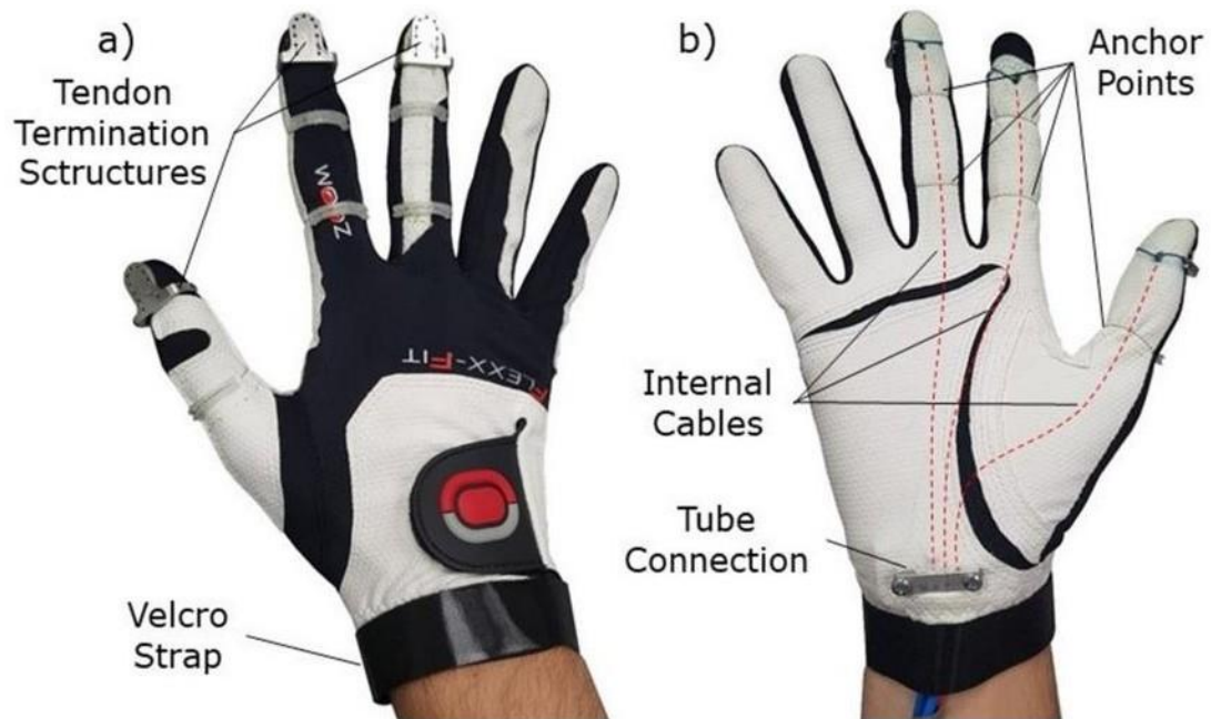
Figure 3.3 Annotated View of the Soft Gloves utilized by the body-powered mechanism[87]
