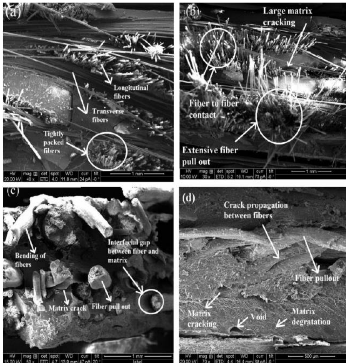
Figure 1.3 SEM Images of tensile fractured specimen of GM/UPR composites (Picture courtesy S. Kalirasu et al., 2015)
