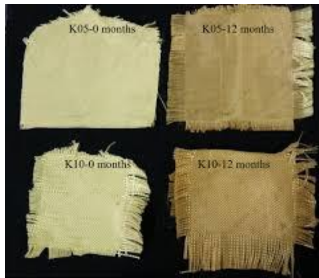
Figure 1.1 Natural ageing effects on the Kevlar Polyaramide fiber (Picture courtesy Victor Hugo Cordeiro et al., 2019)
