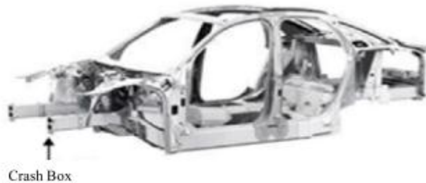
Figure 11: Crash box installation
