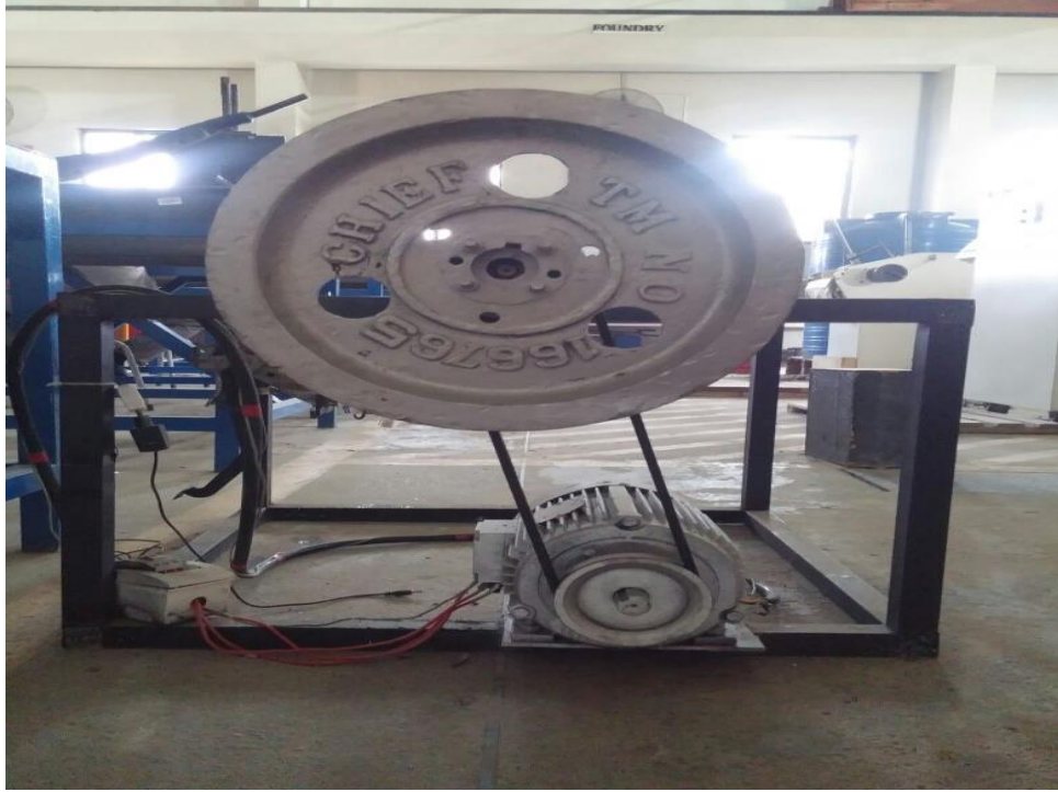
Figure 20: Side View (Flywheel and DC motor)
