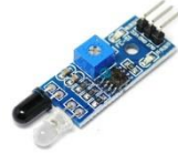
Figure 27: Infrared sensor: To Measure rpm
