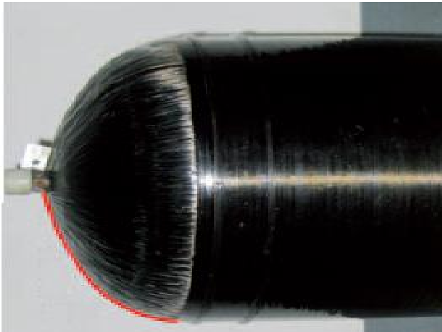
Figure 2.7: Overlapping of the fiber tap
