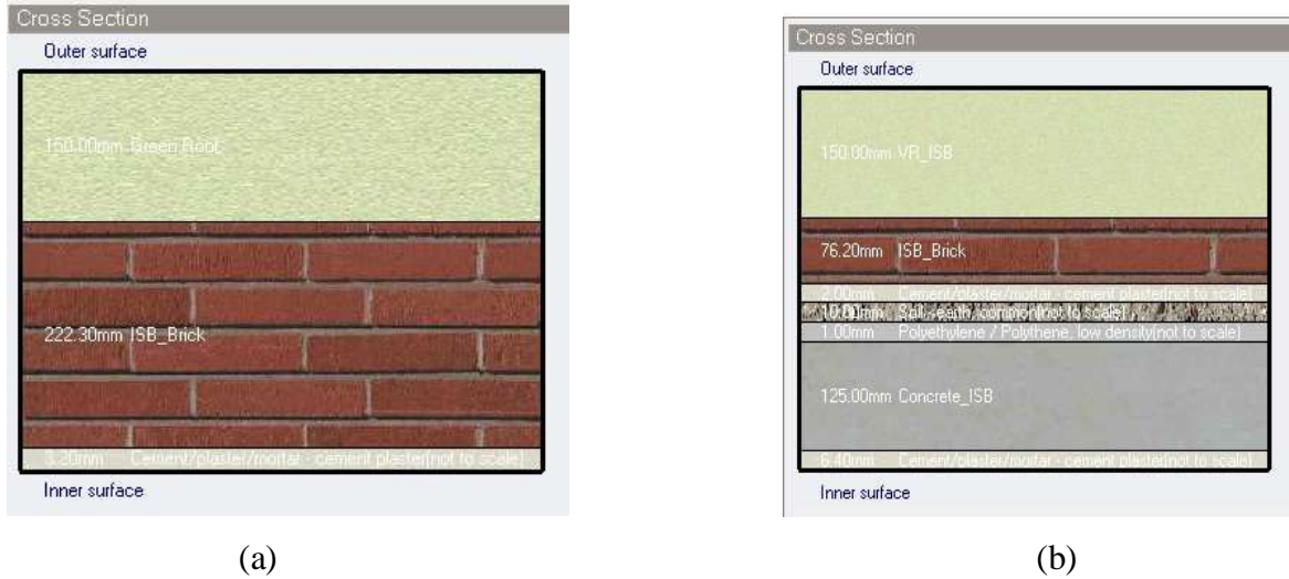
Figure 13(a): design builder layout of green wall (b) layout of green roof
