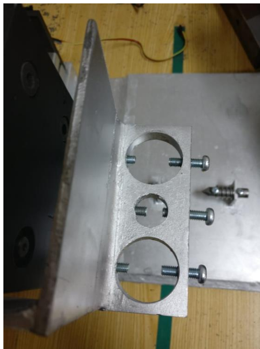
Figure 33 - Holder from the top with corresponding CNC holes and assembled screws
