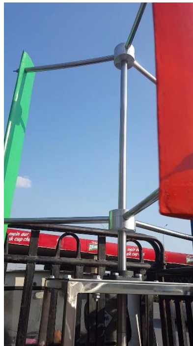
Figure 4.4: Turbine on the load deck of a pickup van
