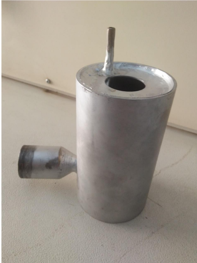
Figure 26 Fire Tube boiler for testing
