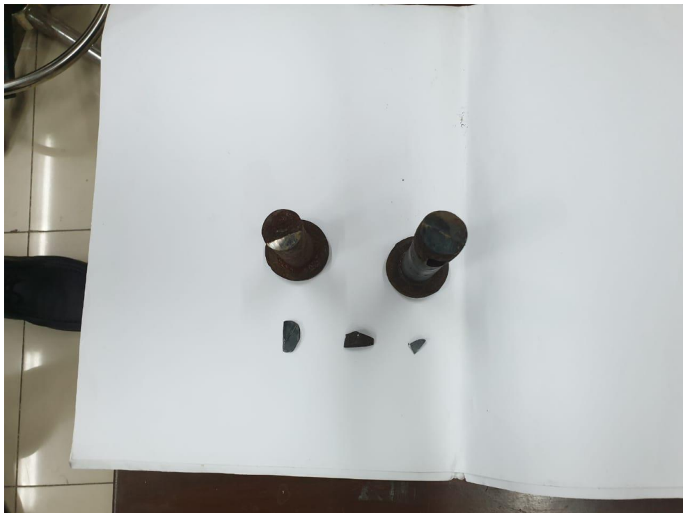
Figure 3.4 Pins and their samples used for the material analysis
