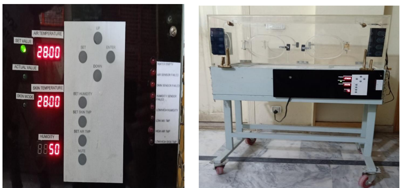
Figure 17: Display of Air, Baby Skin Temperature & Humidity
