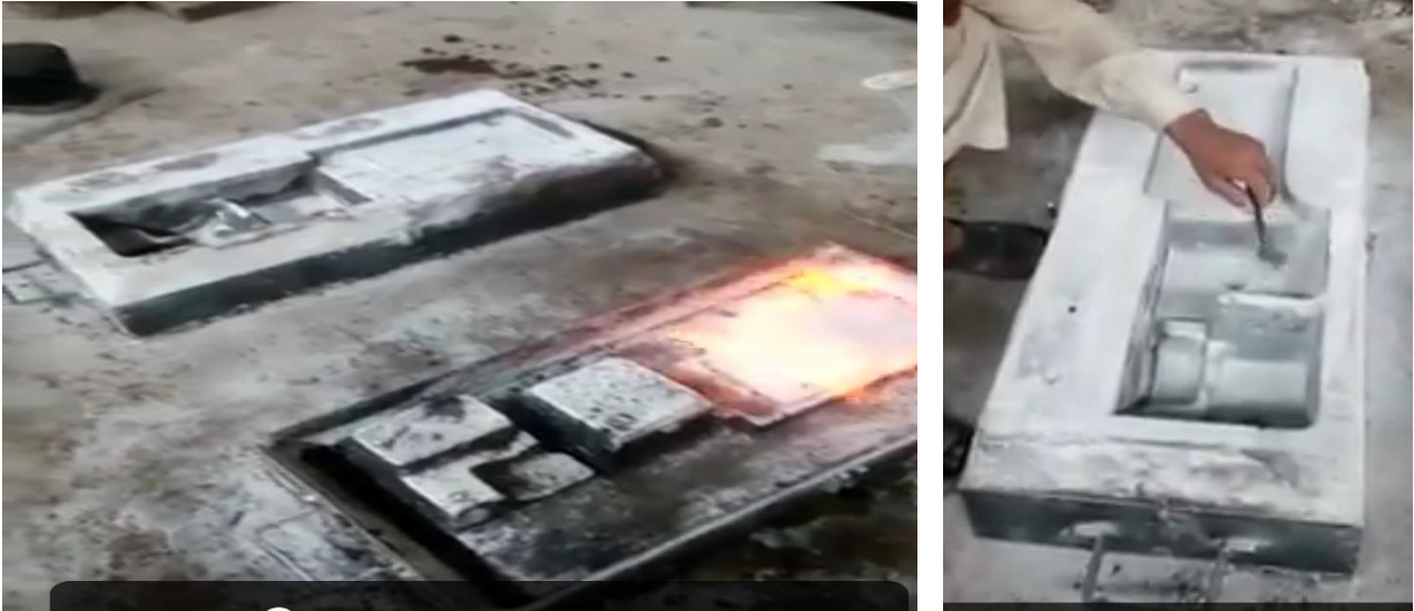
Figure 7: Sand Casting of Core Assembly
