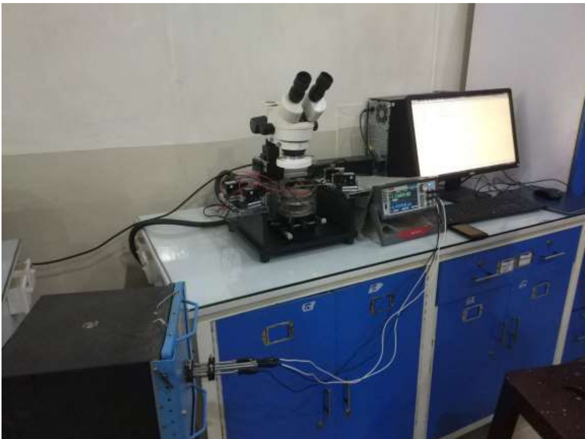
Figure 23: Four Probe Conductivity Test
