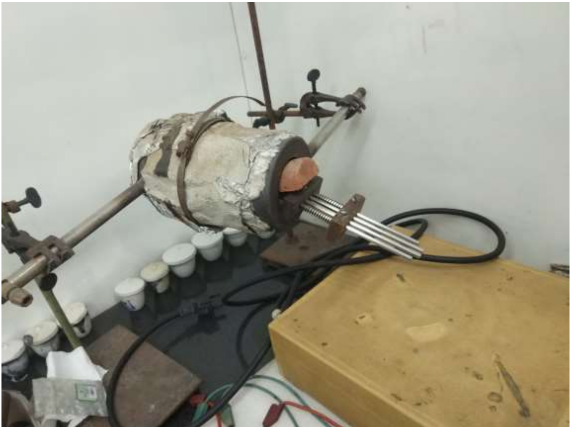
Figure 15: Fuel Cell Furnace
