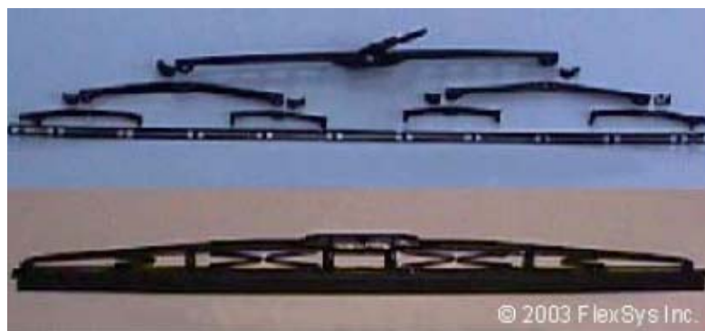
Figure 1.4: Monolithic Windshield wiper developed by Kota group at University of Michigan using compliant mechanisms
