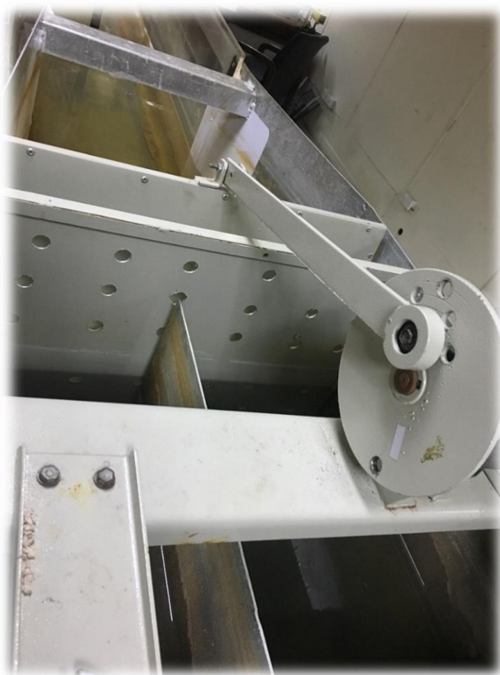
Figure 38: Experimental setup of wave generator with adjustable flapper amplitude
