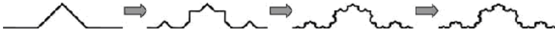
Figure 2.9: First four stages in the generation of Koch fractal curve via IFS approach
