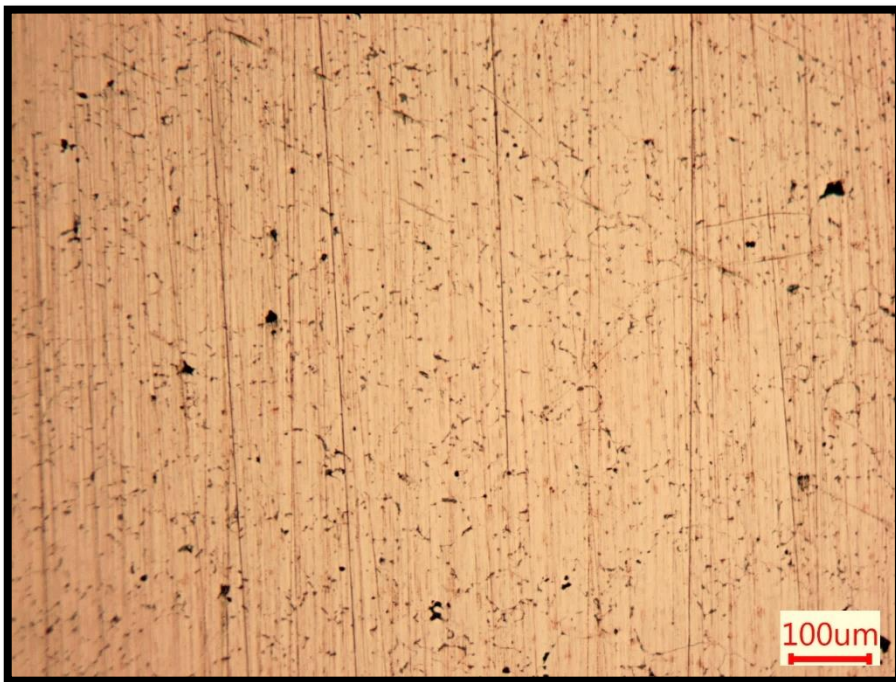
Figure 5. 5 0.2 mm Layer Height Copper Coupon after 45 minutes sintering
