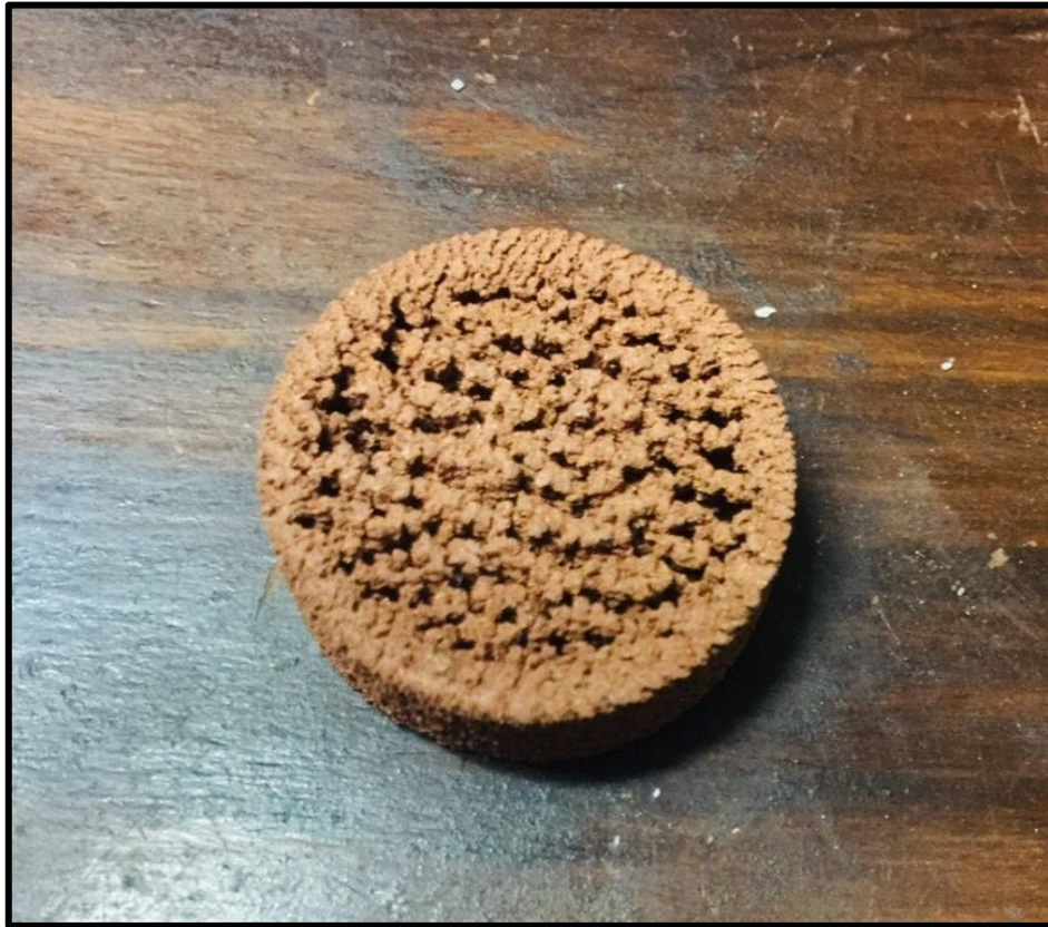
Figure 3. 2: Initial Print with Intermittent Layers
