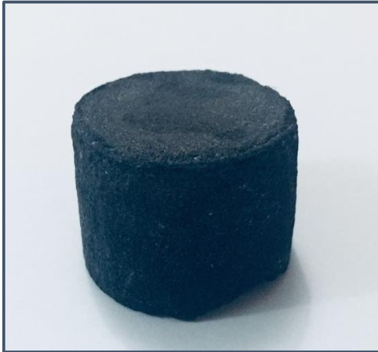
Figure 5. 1: Sintered Sample with External Refractory Ballast Layer
