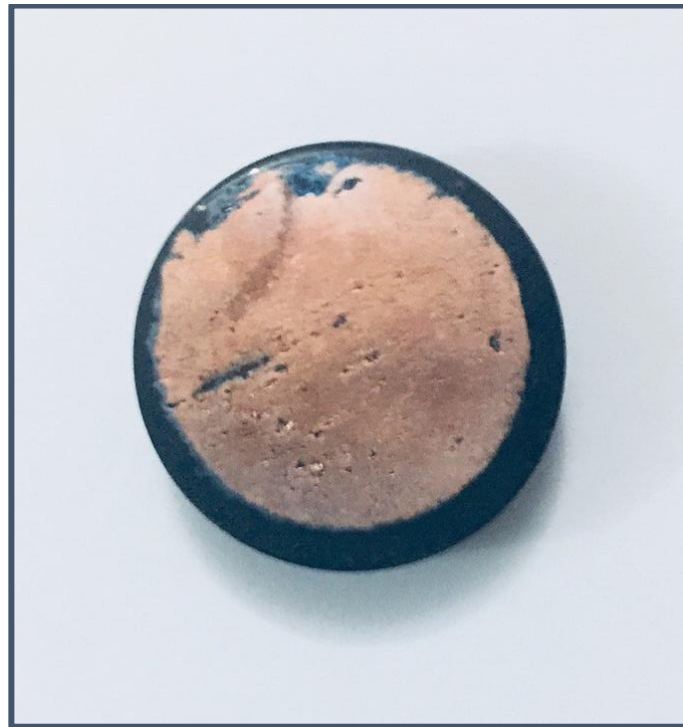
Figure 5. 4: Copper coupon mounted in Bakelite
