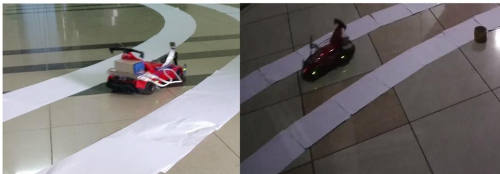
Figure 27: Lane tracking experiment for left-curved track during day and night times
