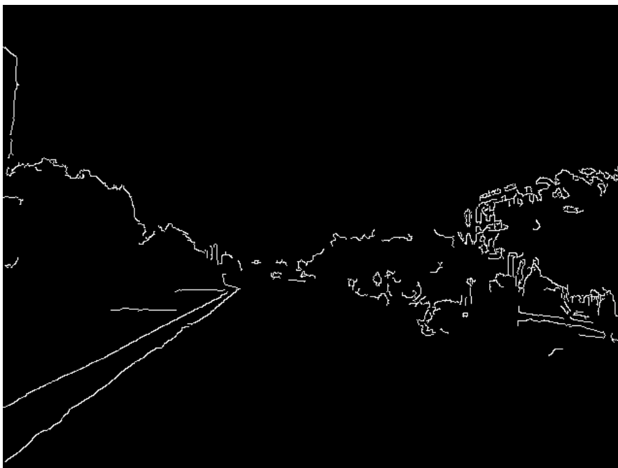
Figure 11: Edges detected by the Canny Edge Detection Algorithm
