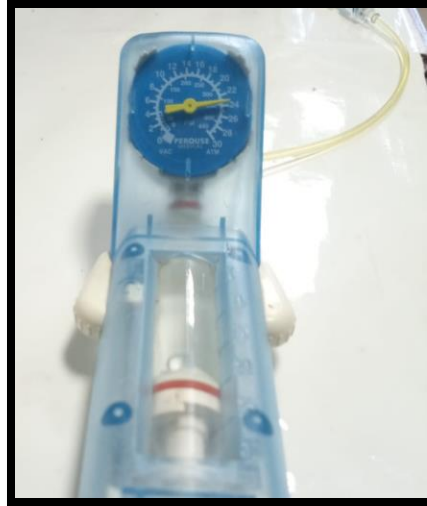
Figure 3.15: The pressure apparatus used for the liquid leakage test
