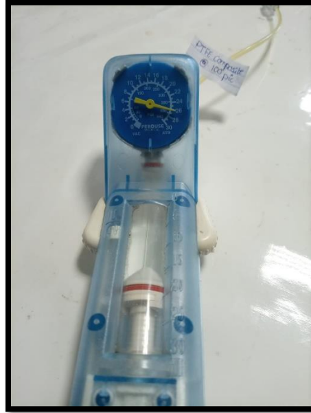
Figure 4.10: Pressure needle didn't deflect back showing the liquid was present in the pump even after 30 seconds.
