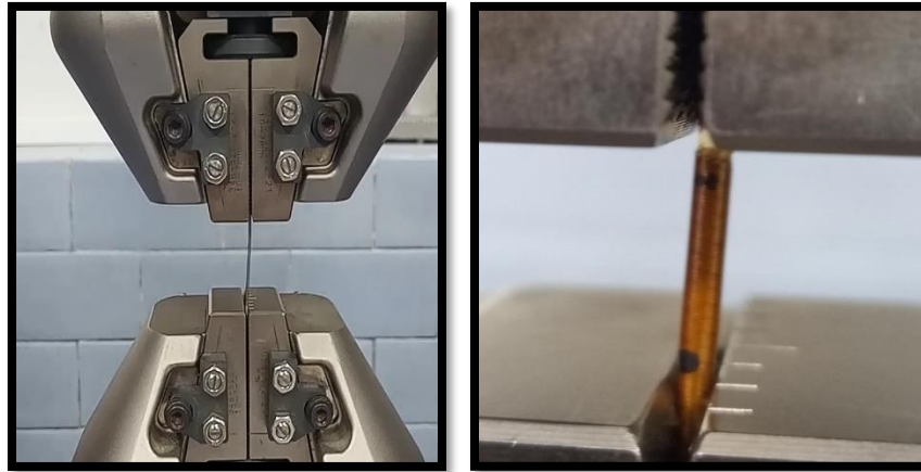
Figure 3.9: Tensile test being carried out on the braided shaft and the guide catheter
