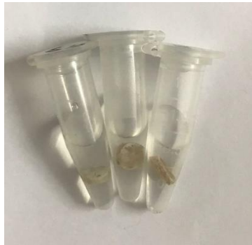
Figure 12: Eppendorf's with 500 µl diluted culture and immersed composite discs immersed
