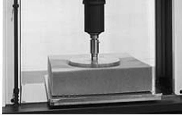
Figure 3.5: Compression testing apparatus
