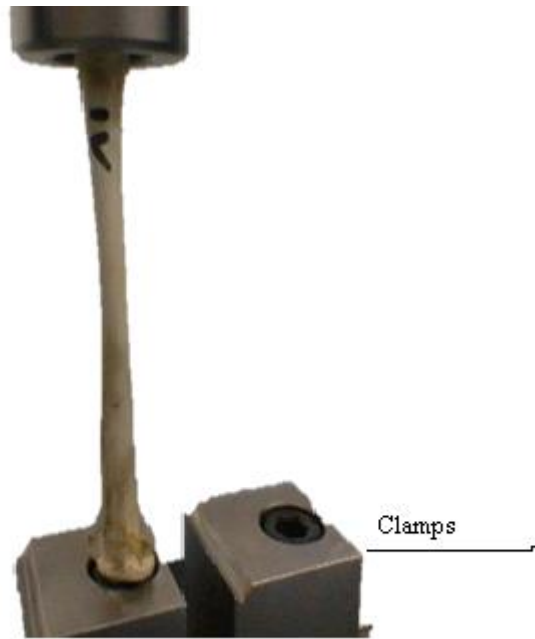
Figure 3.6: Sample during mechanical testing (Axial Compression being applied to the bone).
