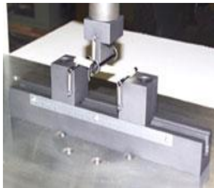
Figure 3.4: 3-Point bending apparatus
