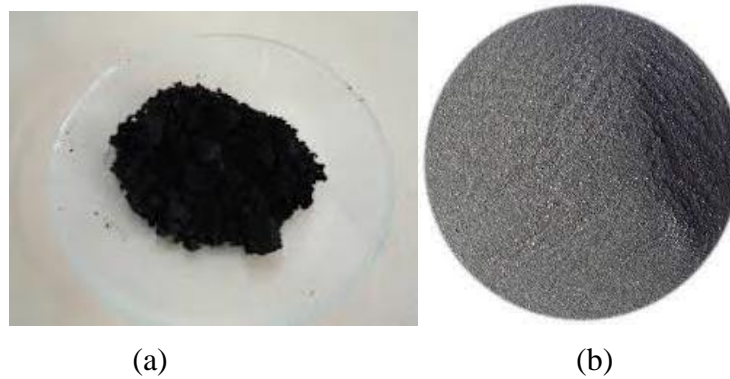
Figure 0.17 (a) Magnetic powder for the magnetite ( \text{Fe}_3\text{O}_4 ). (b) Iron particles collected after laser cutter machine we use these particles as microrobot in our experiment
